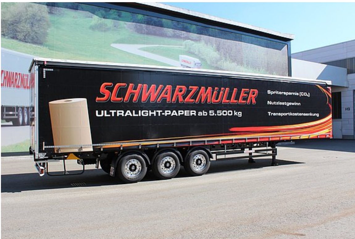
3-axle lightweight sliding tarpaulin platform semitrailer - paper rolls
