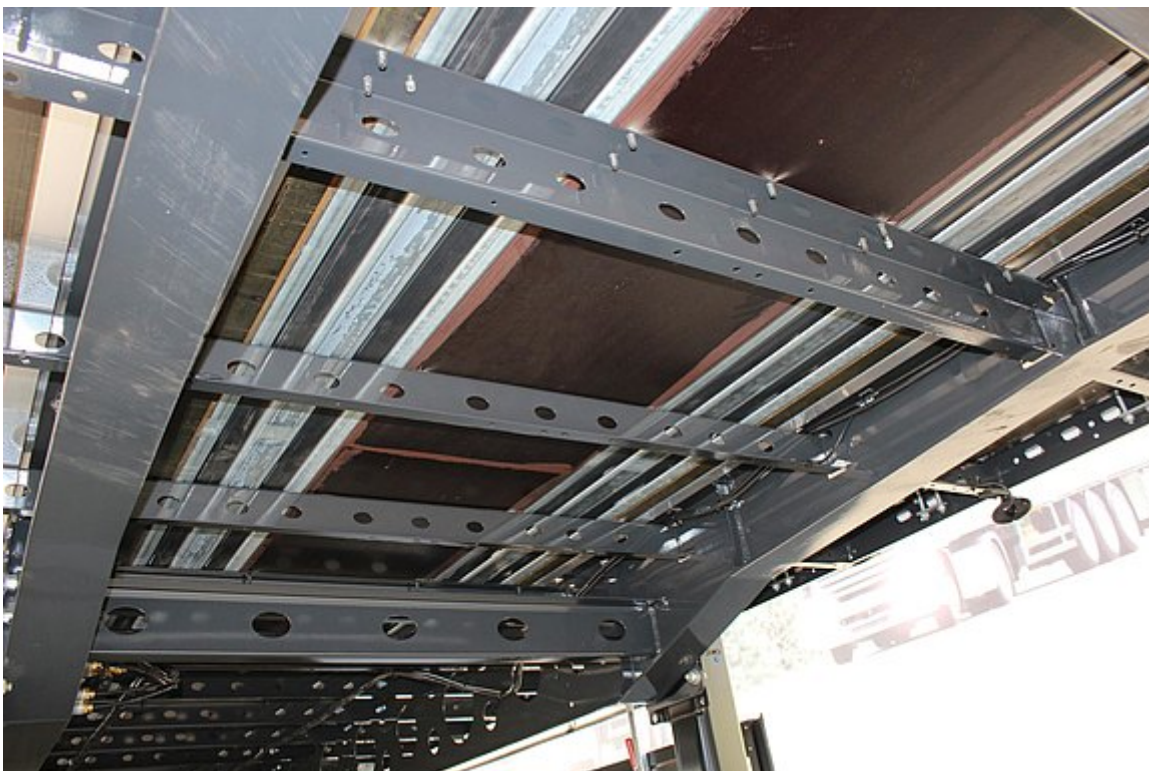
27-mm resin-coated panel floor, alongside side members and with 12-mm resin-coated surface on top, rear 300 mm made from aluminium button sheet 7/9 mm, flush with external frame (7 t stacker axle load according to CSC)
