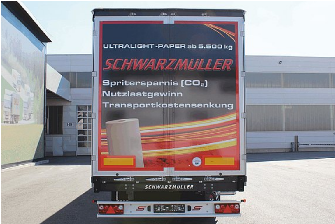
Bolted portal at rear with aluminium corner posts and fully opening double door
