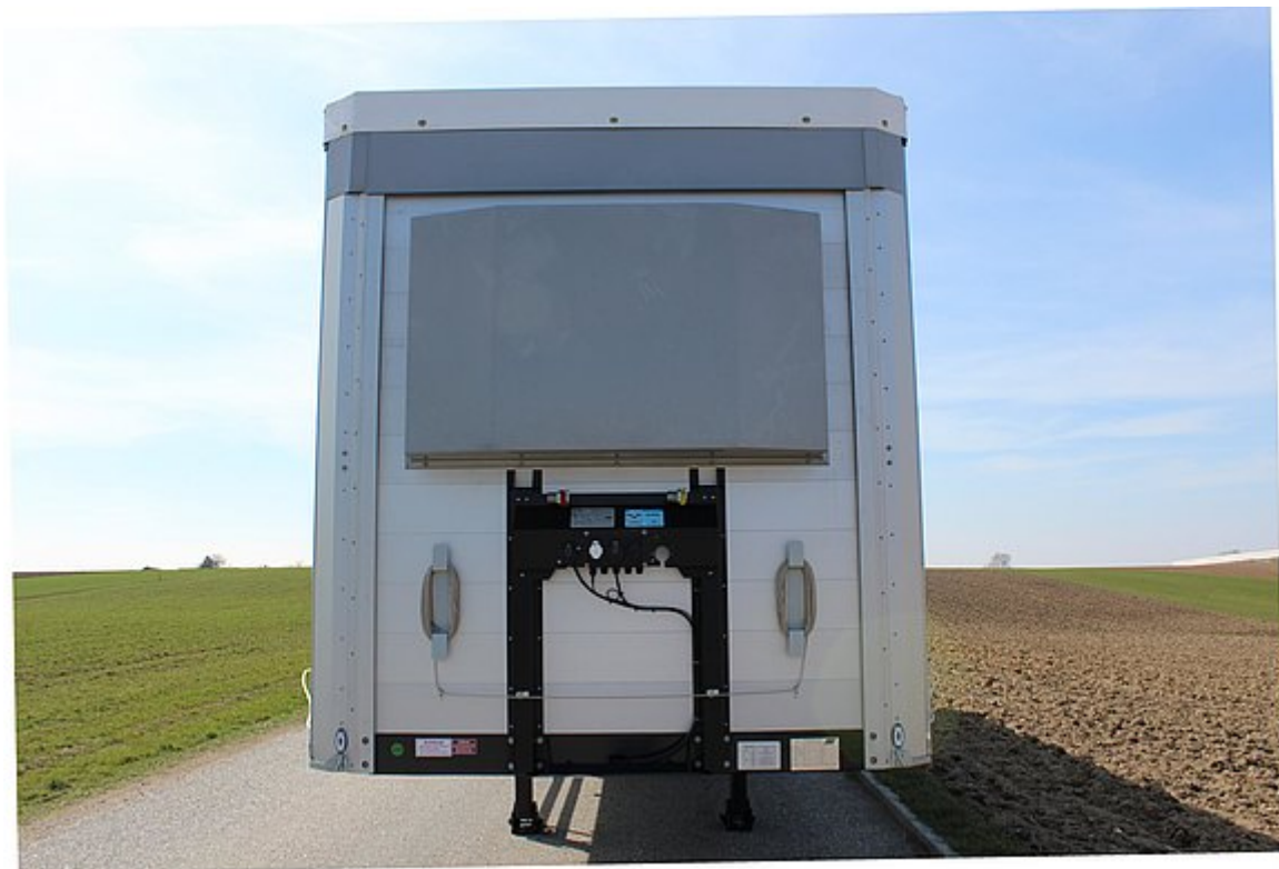
Wedge box on front wall with space for wedges, pallet rollers, lashing straps and non-slip mats
