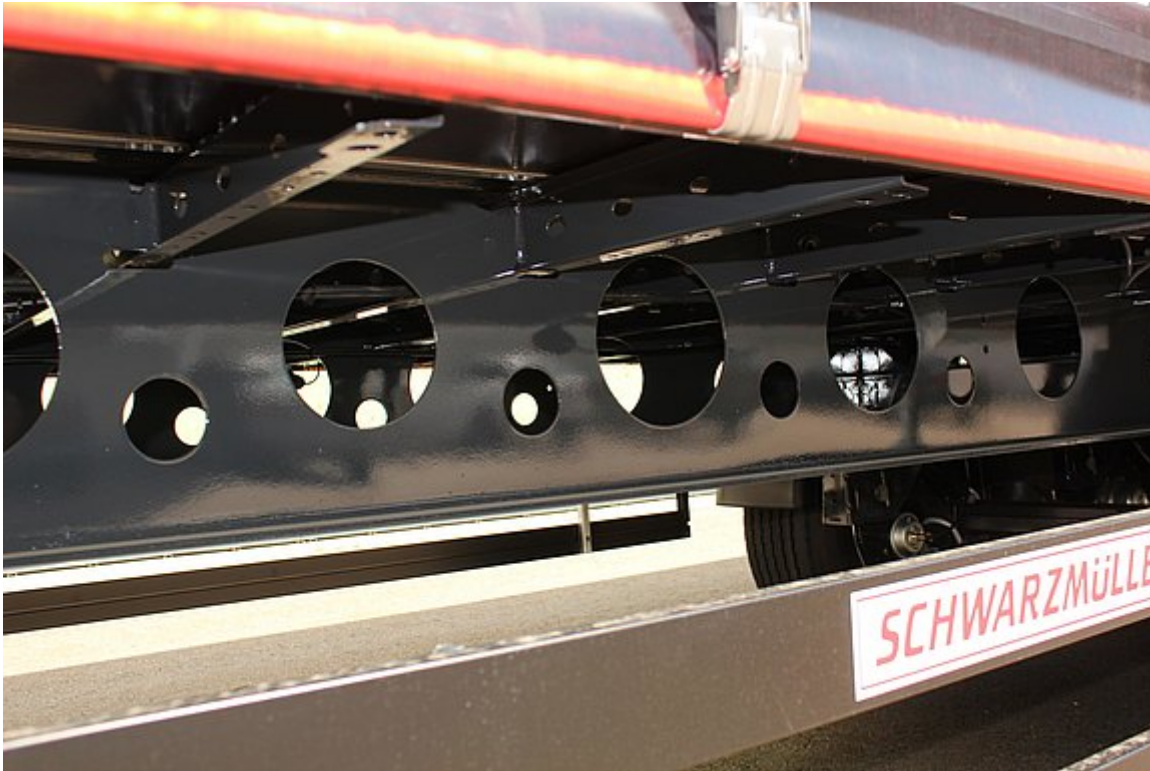
Lightweight construction with perforated side members made from special high-strength Naxtra steel
