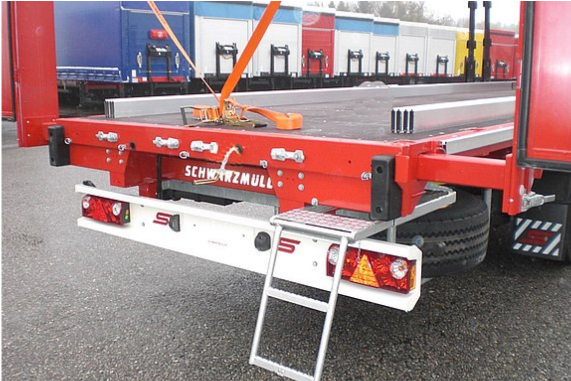
OPTIONAL: Extendible portal columns (each by approx. 400 mm) for easier loading and unloading
