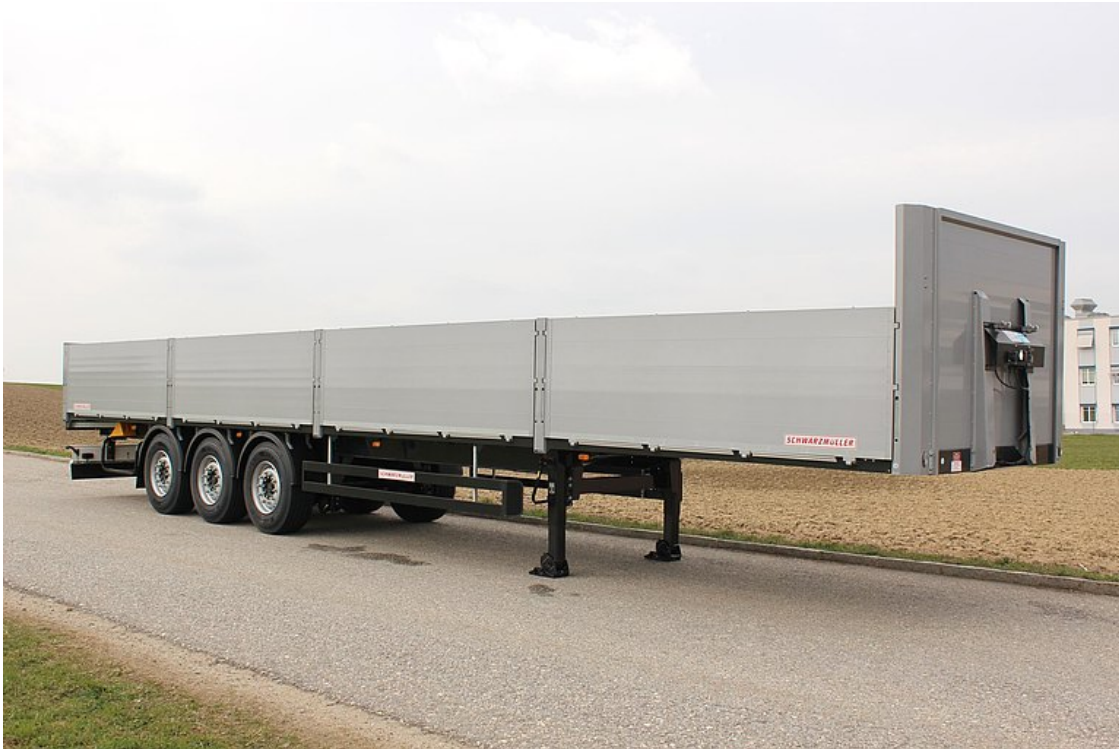
Reinforced body design with load securing certificate in accordance with DIN EN 12642 Code XL
