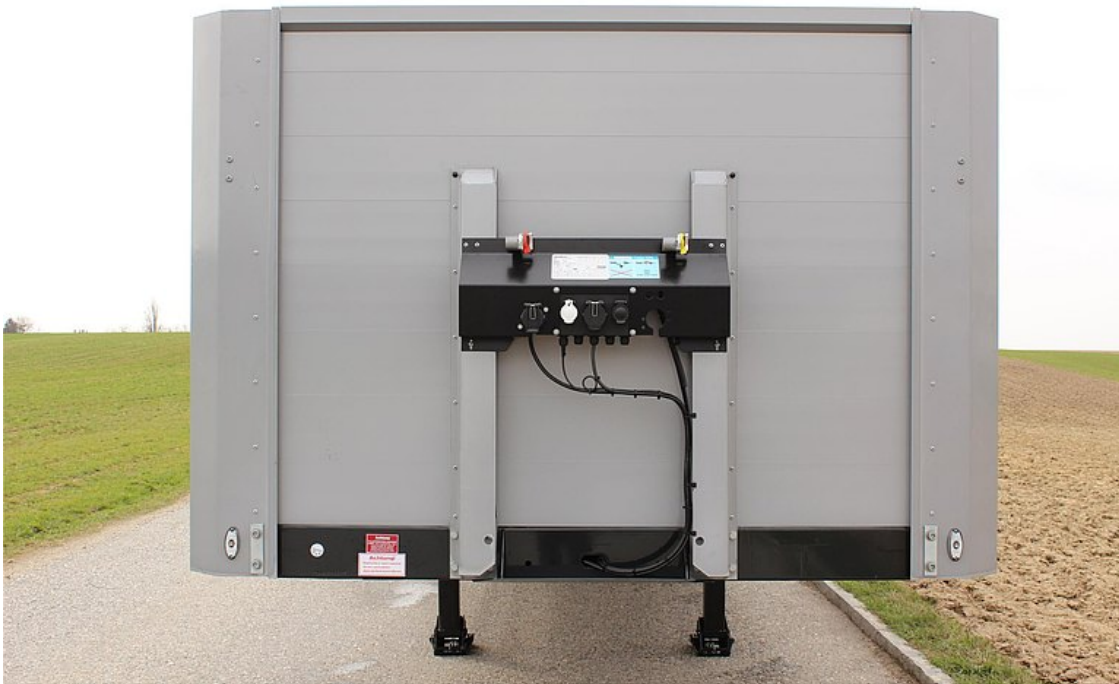
Fixed aluminium hollow profile front wall with 2 centre supports, inside with 2 lashing eyes for load securing and reinforced with steel sheet
