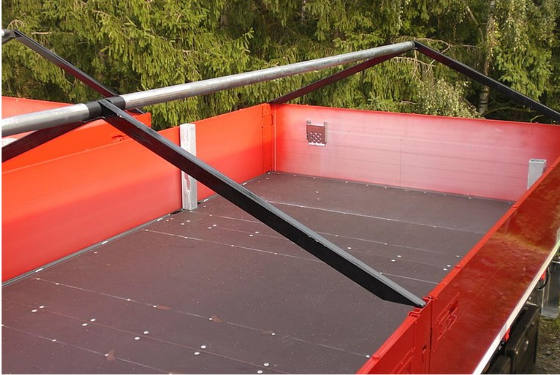
OPTIONAL: Cement cover - 4 roof arches directly inserted into the central and rear corner posts and 1 central row of roof planks (roof inclination 500 mm)
