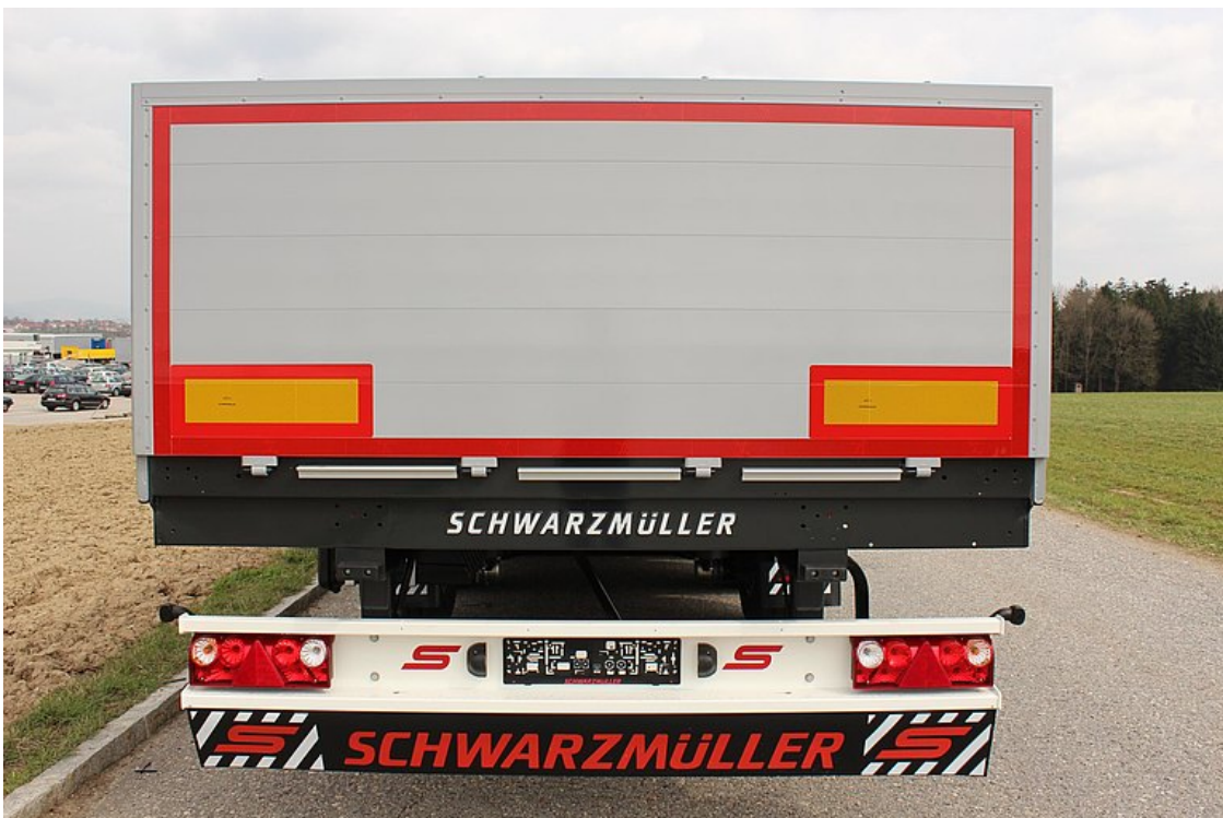
Foldable aluminium hollow profile rear wall, with rubber seals on the horizontal and vertical planes
