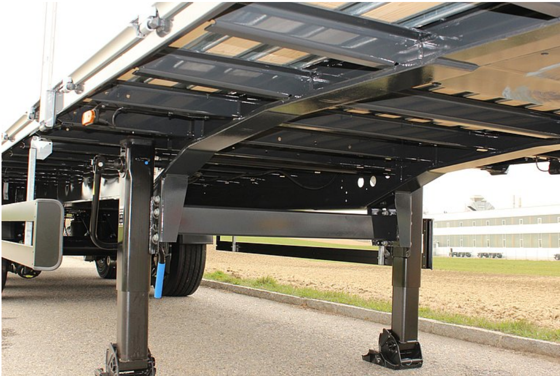
Reinforced frame design for point loading 20 t on 4 m in the centre of gravity
