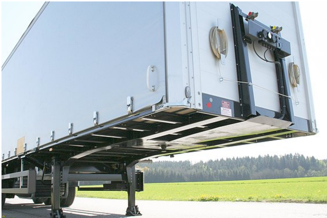
Torsionally rigid, welded ladder frame structure
