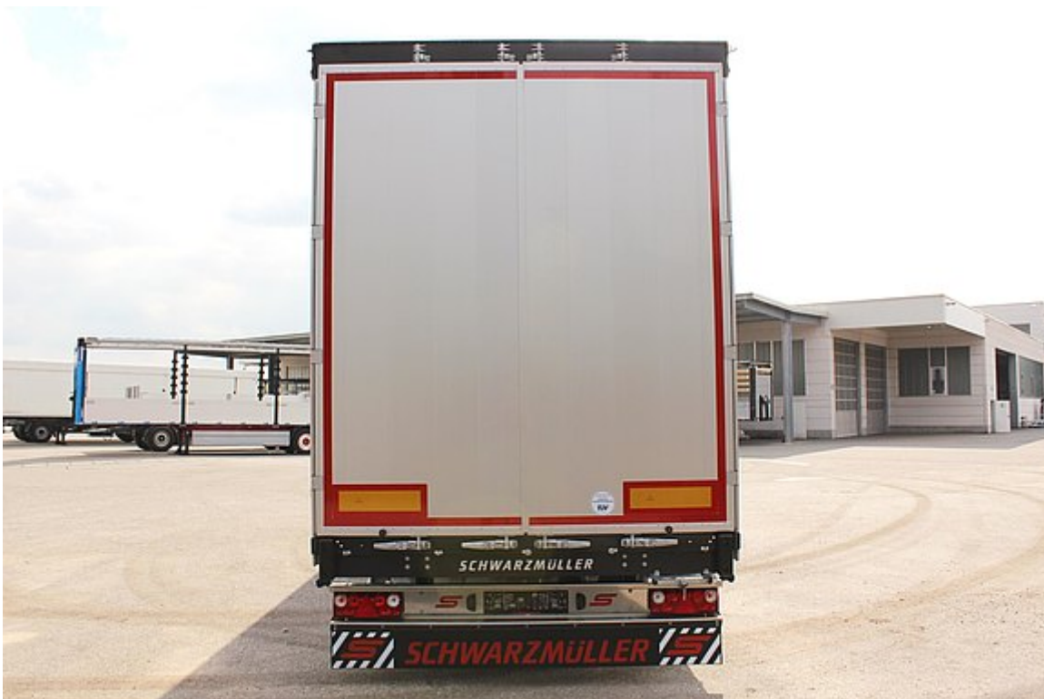
Portal bolted onto the rear with aluminium corner posts incl. fully opening double door in profile design
