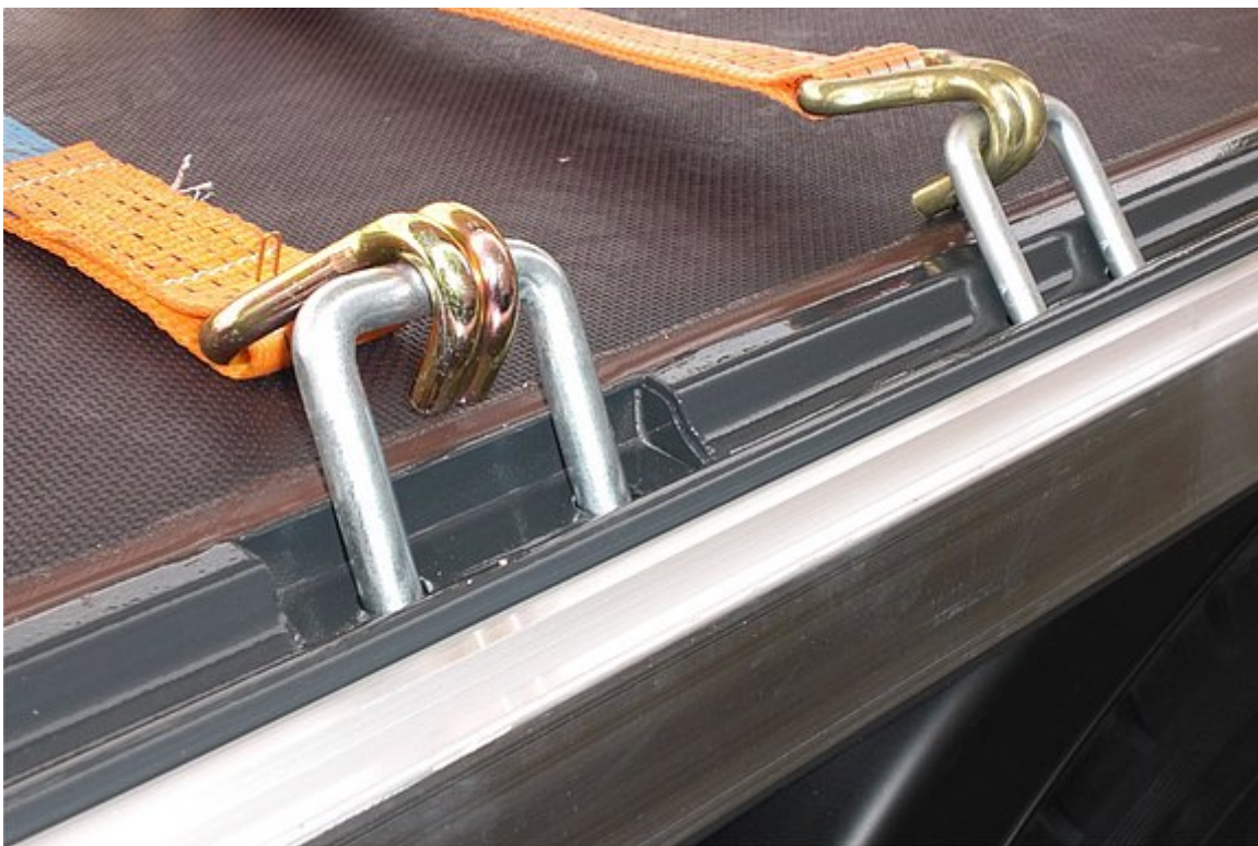
External frame with 23 pairs of recessed 2.5 t lashing points and an additional 5 pairs of 4 t lashing points in the recess area
