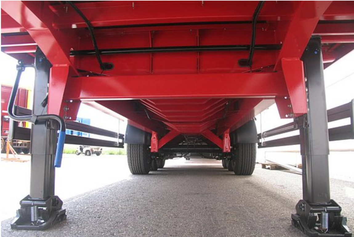
Reinforced frame construction for coil transports of 30 t at centre of gravity across minimum of 2,000 mm load length
