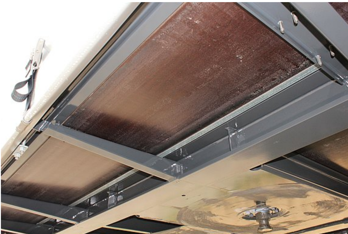
27 mm resin-coated panel flooring, flush with external frame
