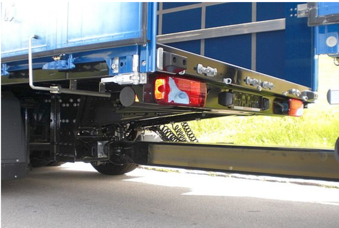
Special tow attachment for low-clearance, central axle trailers
