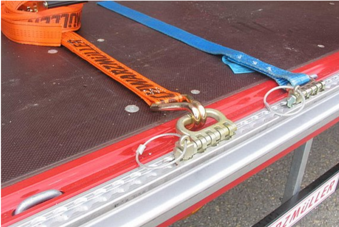
OPTIONAL: Variable load securing via bolt-on lashing systems, such as: airline lashing rail
