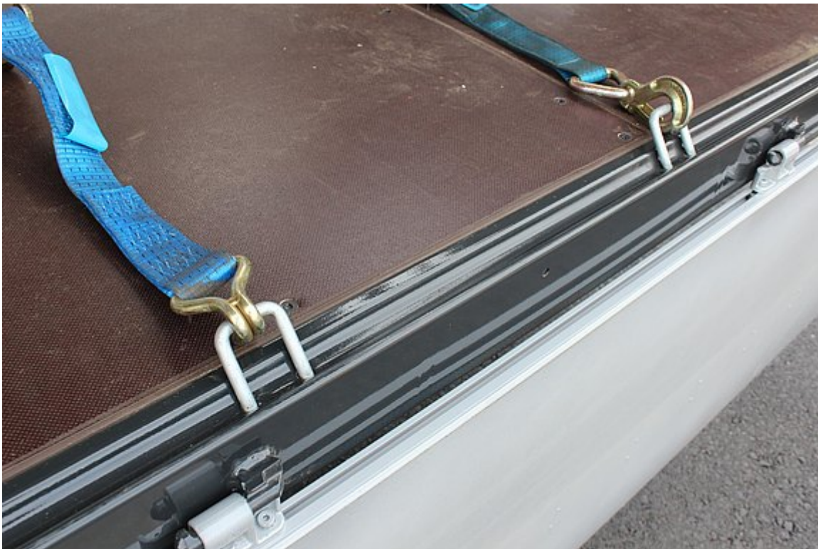
External frame with recessed 2.5 t lashing points
