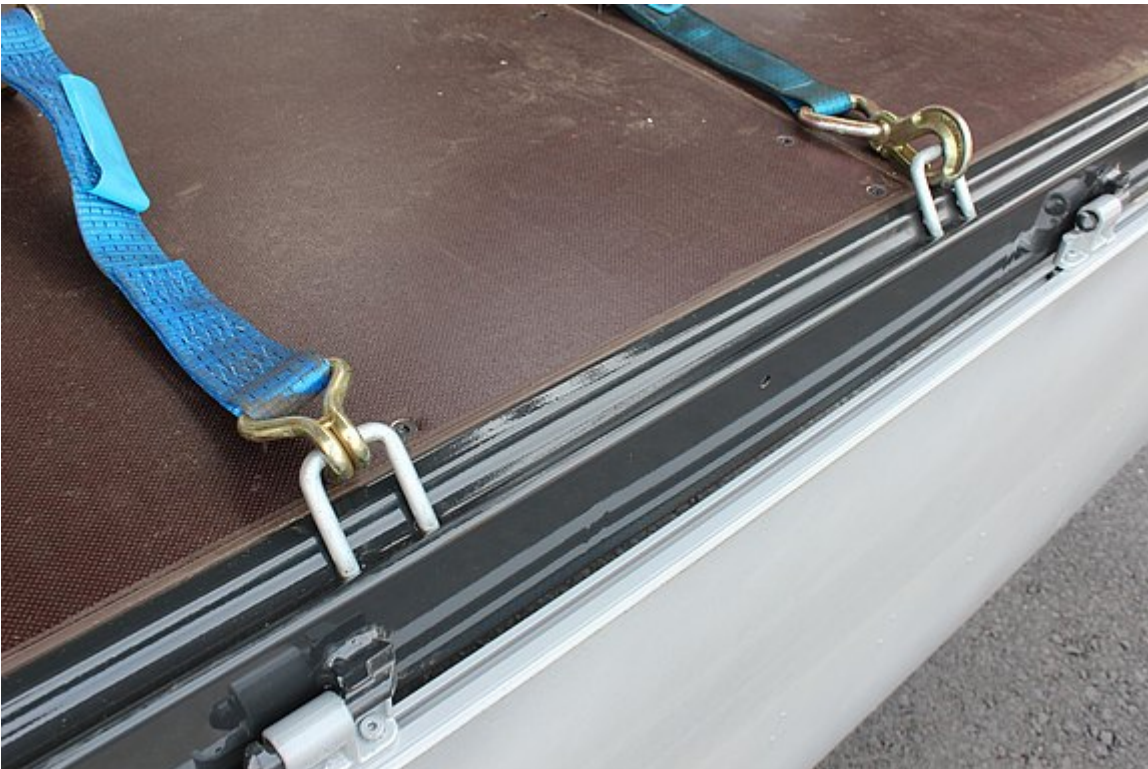
External frame with recessed 2.5 t lashing points
