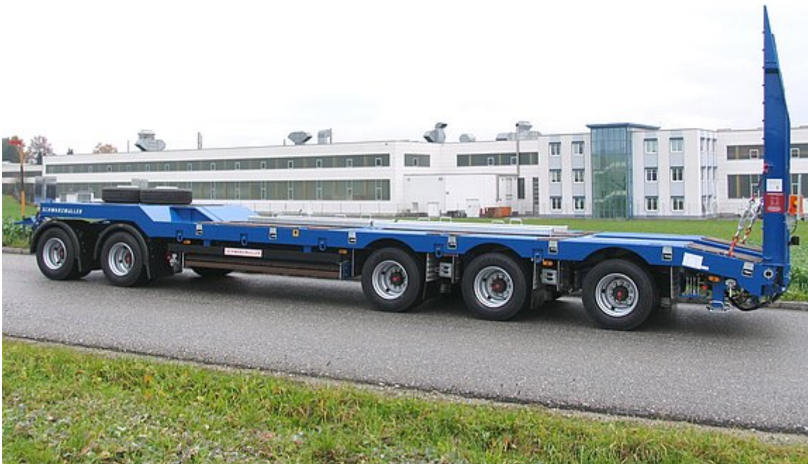
5-axle low loader trailer with offset platform
