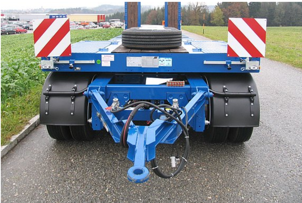
Front offset platform with accessory compartments and pull-out warning signs for transporting
