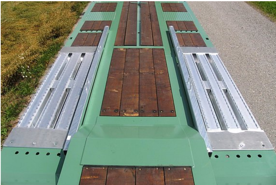
Wheel recesses with drive-on aluminium cover
