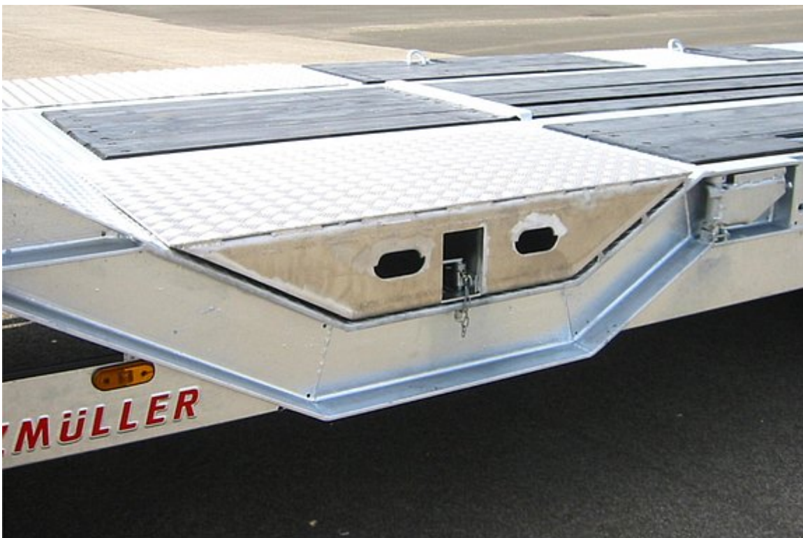
Wheel recesses in different designs for transporting special construction vehicles
