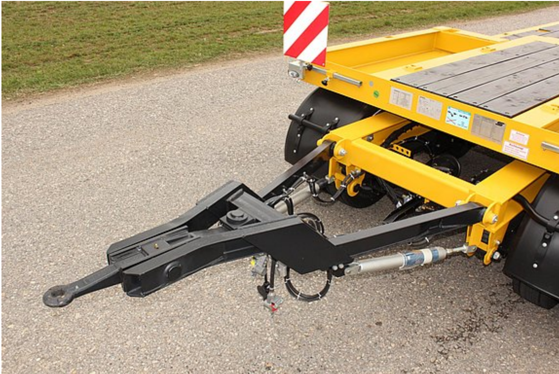
OPTIONAL: Offset drawbar with pivoting eye, 40 + 50 mm
