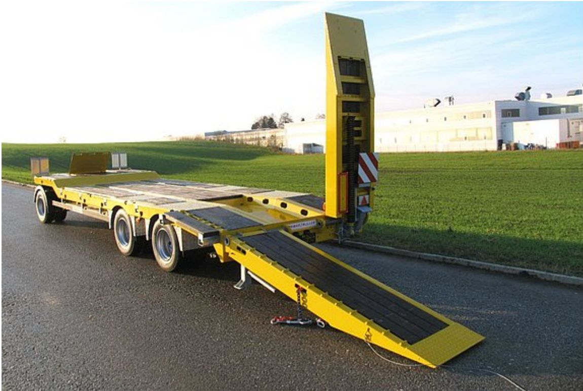
2 folding single-part loading ramps with hardwood flooring
