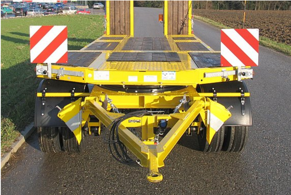
Bogie at front incl. drawbar and pull-out warning signs on frame for transporting wide loads
