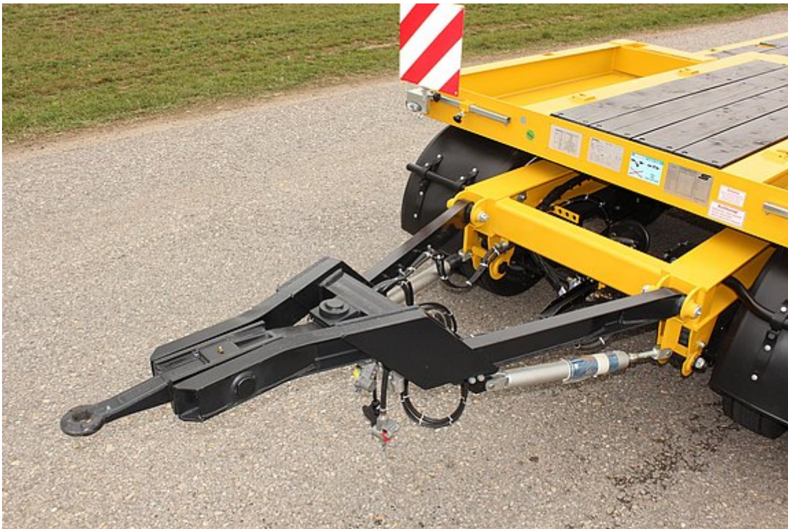
Offset drawbar with pivoting eye, 40 + 50 mm
