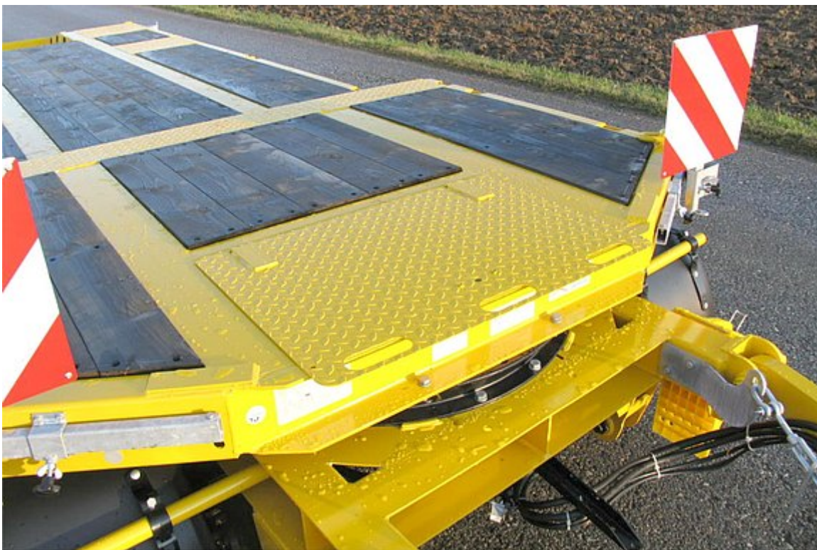
Front offset platform with accessory compartment including lid
