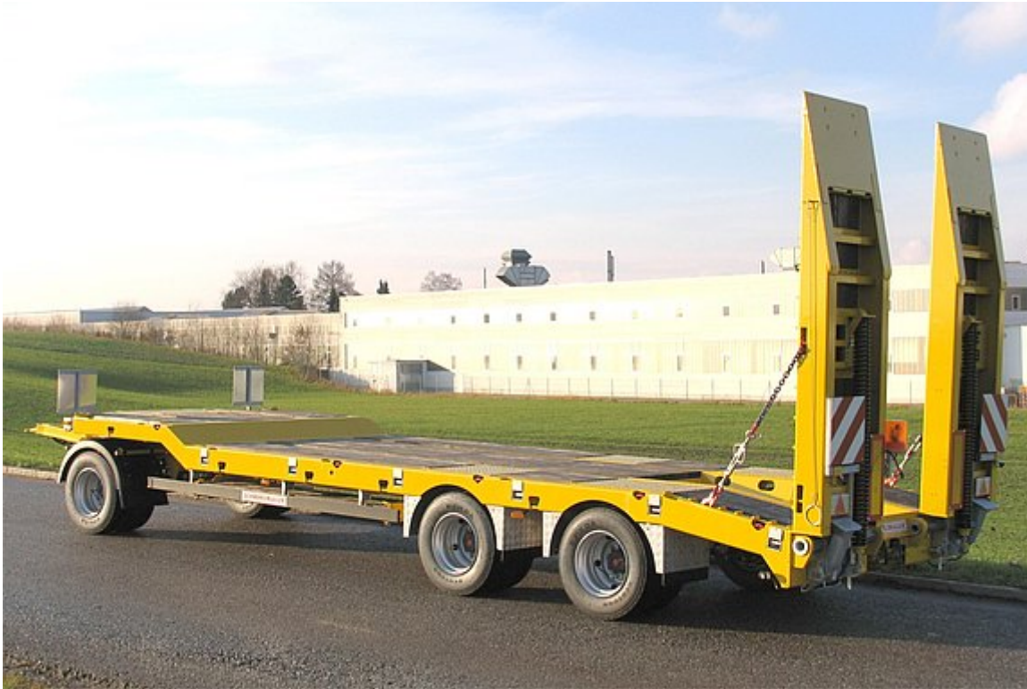
3-axle low loader trailer
