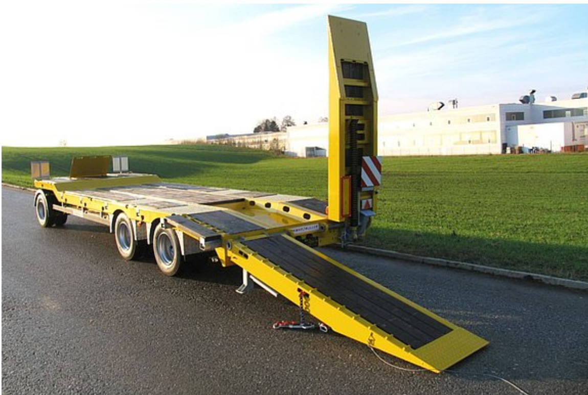
2 folding single-part loading ramps with hardwood flooring
