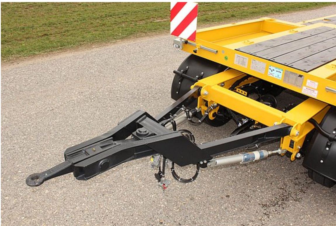
Offset drawbar with pivoting eye, 40 + 50 mm
