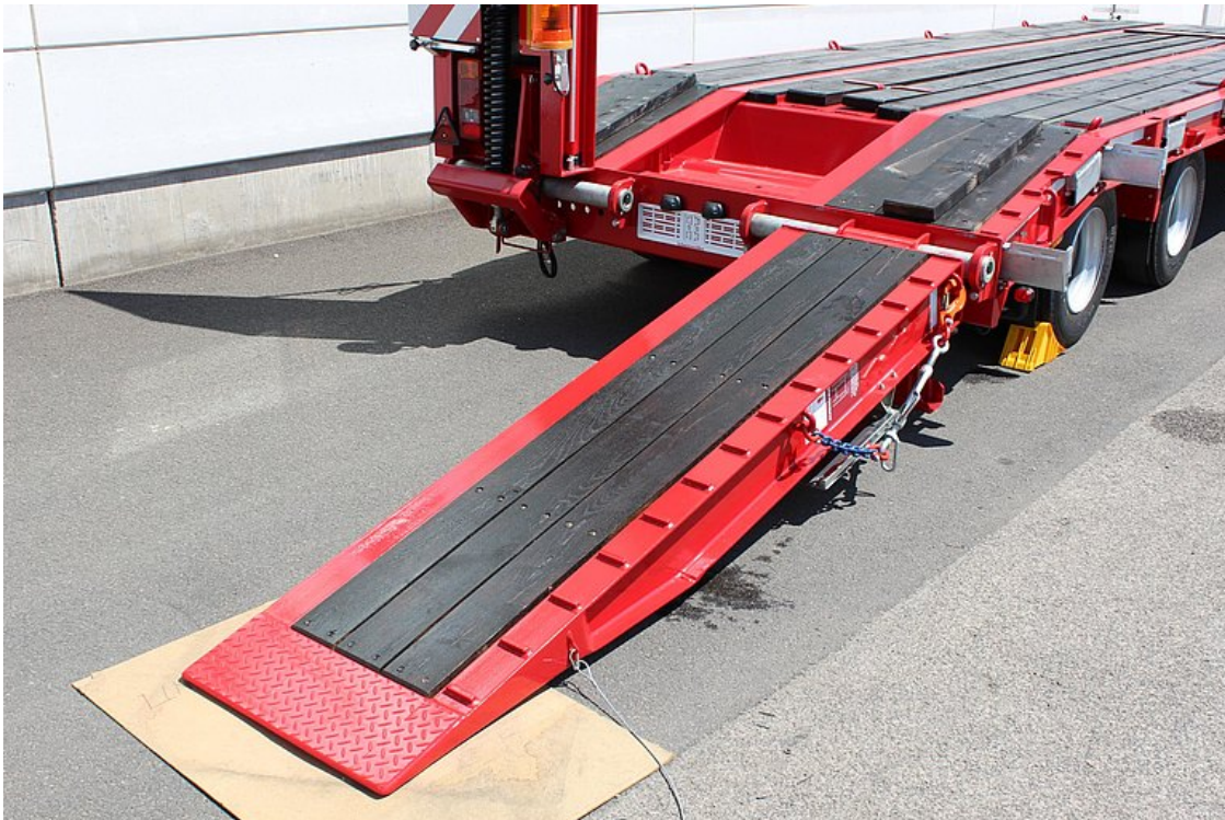
Loading ramps with hardwood flooring and welded square ribs
