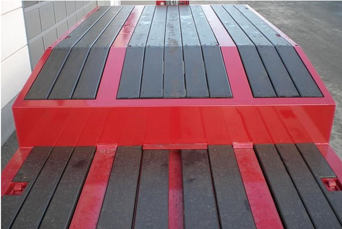
Drop-deck area and offset platform with softwood flooring
