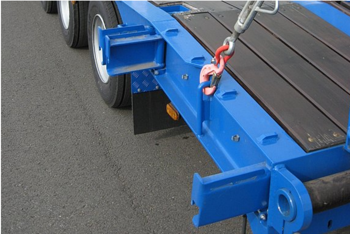
Foldable, pivoting extensions, incl. extension planks for transporting wide loads
