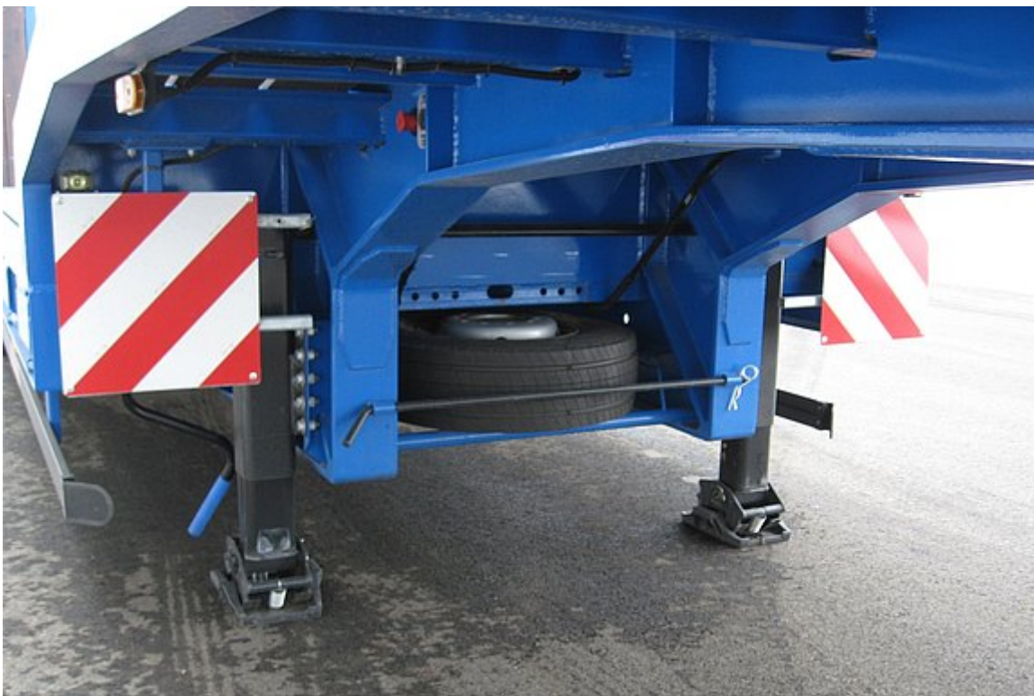
Welded steel construction - high point loading due to narrow cross member spacing
