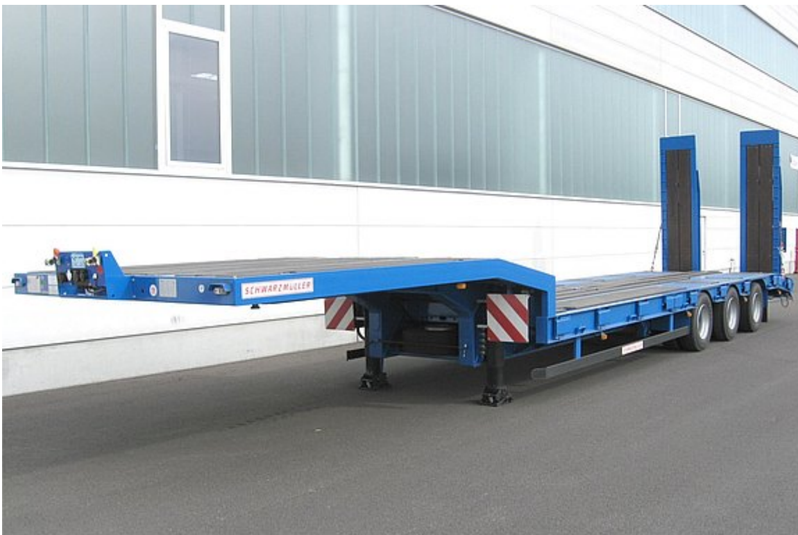
3-axle low loader semitrailer
