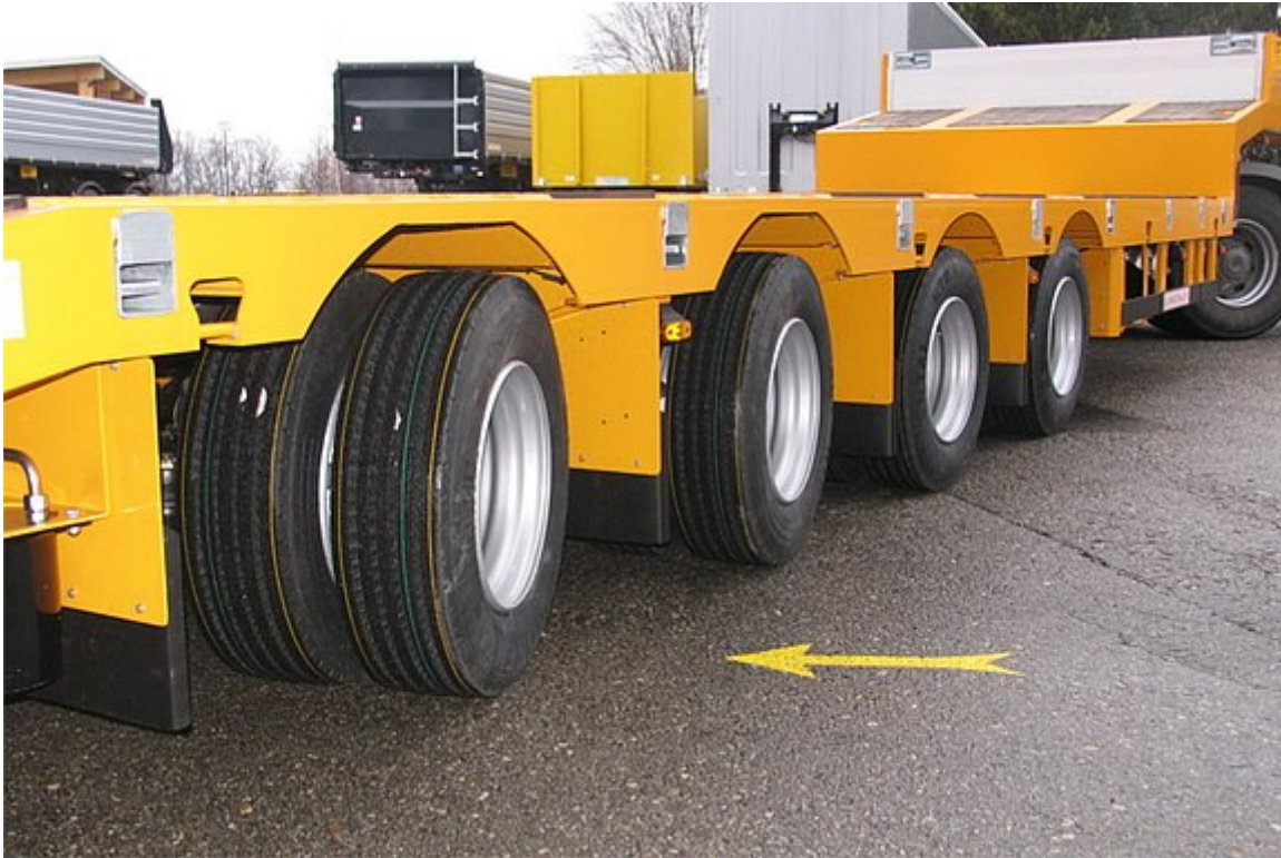
Third and fourth axles are steered trailing axles for improved cornering and lower tyre wear
