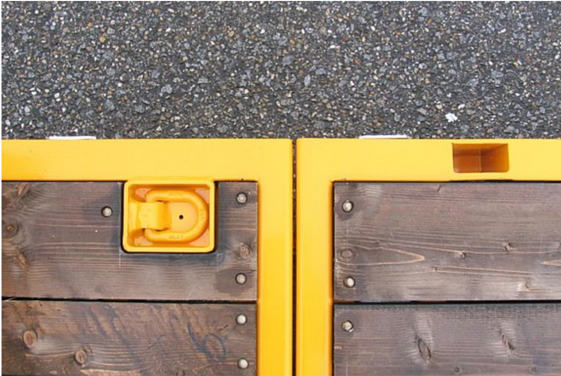
Recessed, folding, floor-mounted lashing eyes in the drop-deck section and lashing points in the external frame
