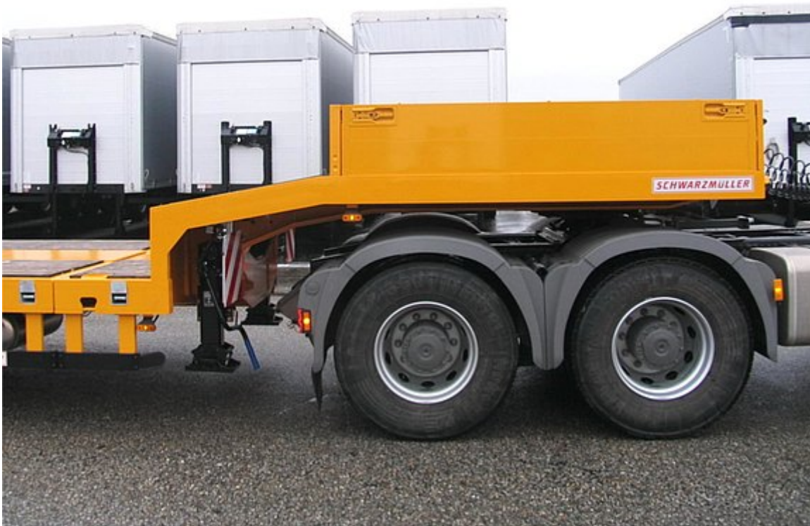
Offset platform raised at the front, incl. plug-in side walls
