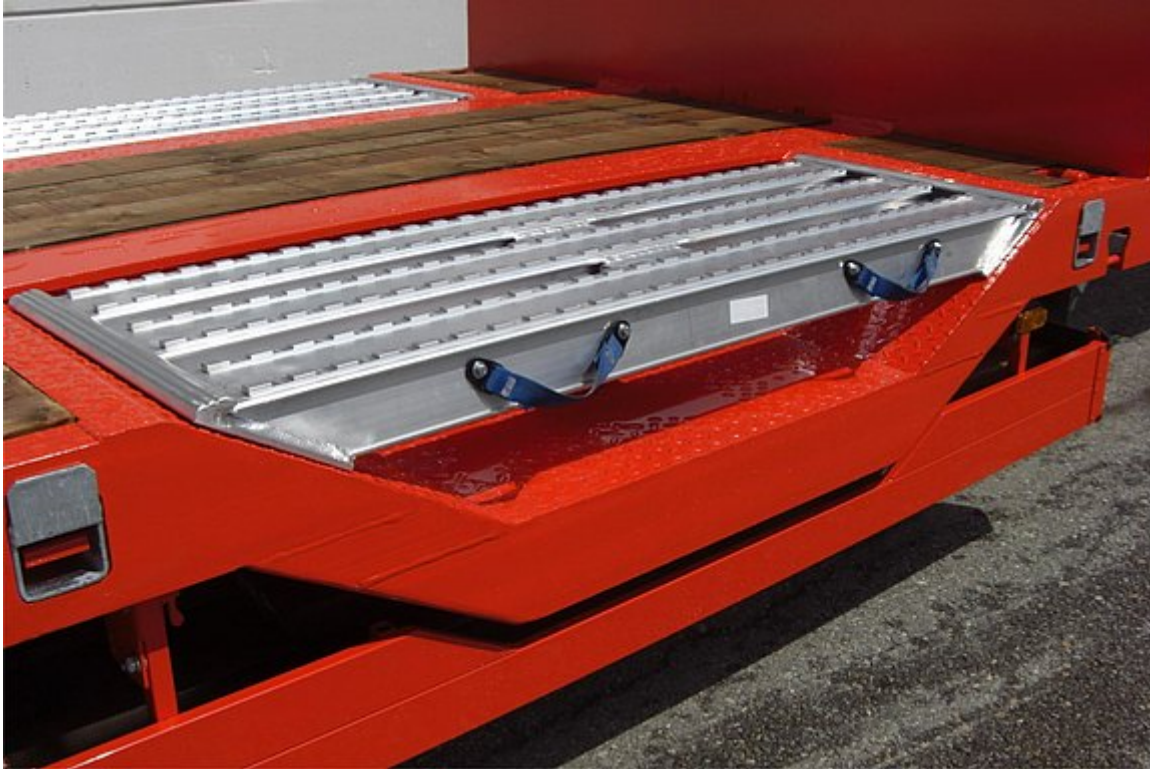
OPTIONAL: Wheel recesses for transporting special vehicles
