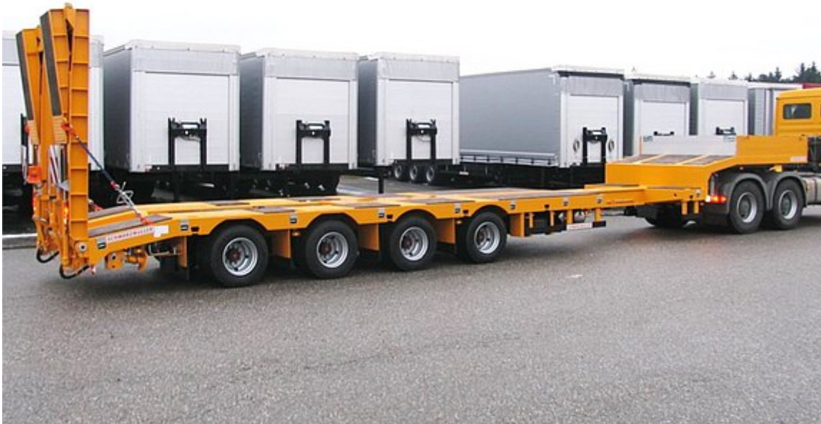
4-axle low loader semitrailer - reinforced - extendible
