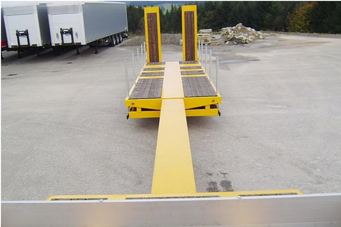
Drop-deck loading platform with softwood floor and tubular posts in external frame
