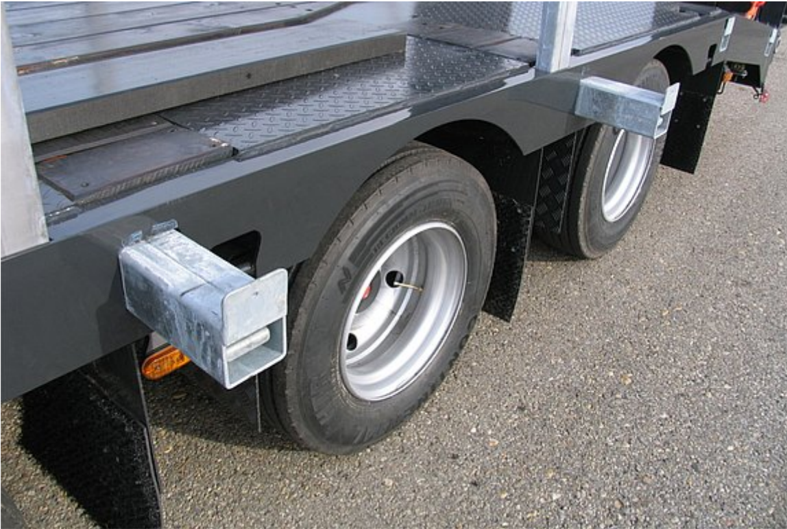
Pull-out extensions incl. extension planks for transporting wide loads
