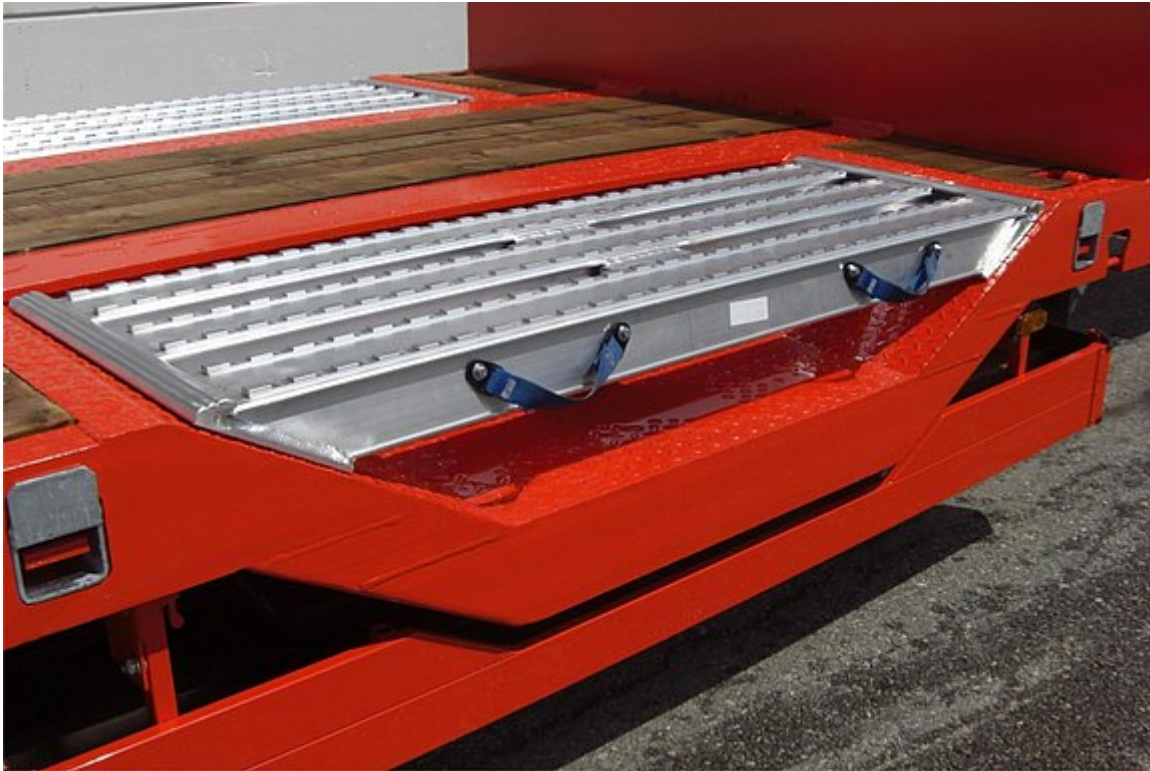
OPTIONAL: Wheel recesses for transporting special vehicles
