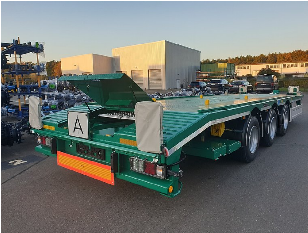
Special equipment with stanchion storage boxes and wide load signs
