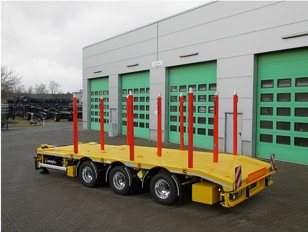
EXTE stanchions special equipment, trailing steering axles and aluminium rims
