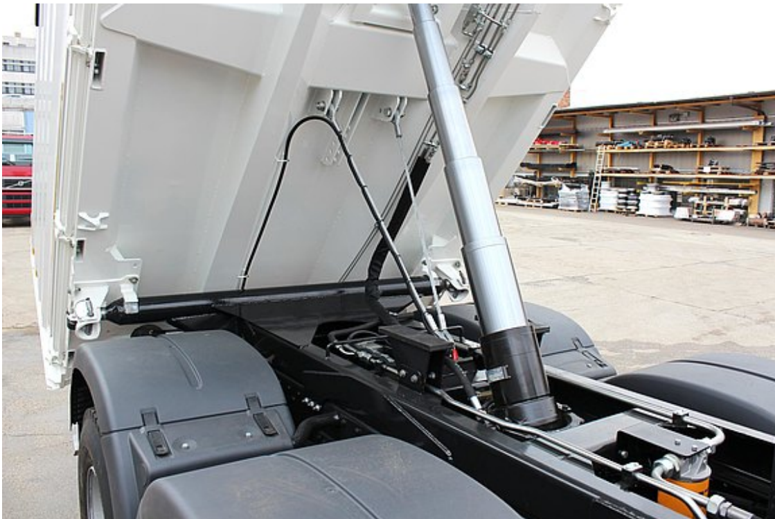
Hard chrome-plated, high-quality tilt cylinder
