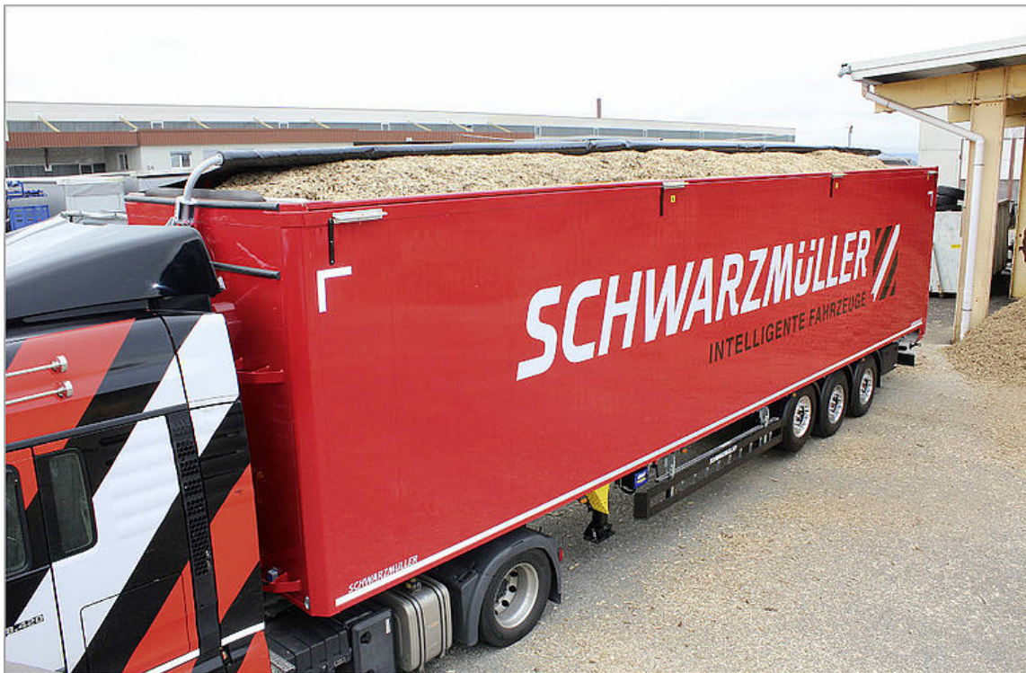
3-axle sliding floor semitrailer with aluminium frame - optional: with electric roller cover
