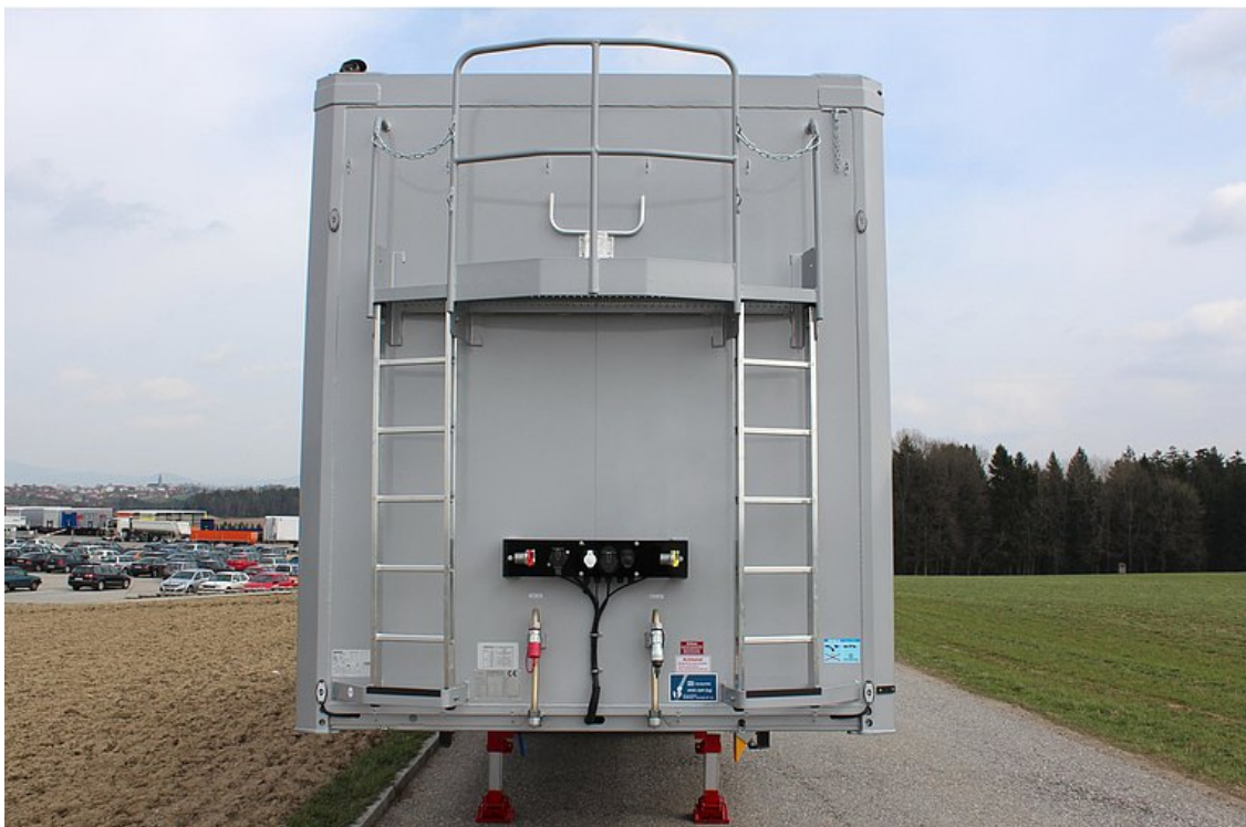
Aluminium hollow profile front wall, fixed with upper stabiliser frame
