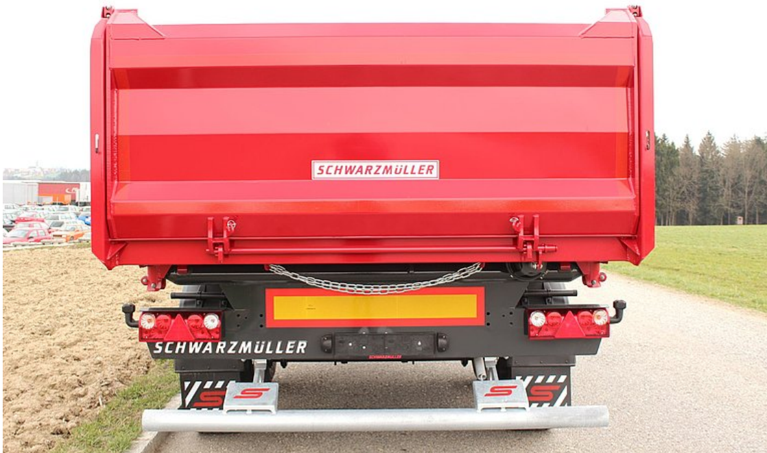
Steel sheet rear wall, hinged with raised bearing and autom. pneumatic lock
