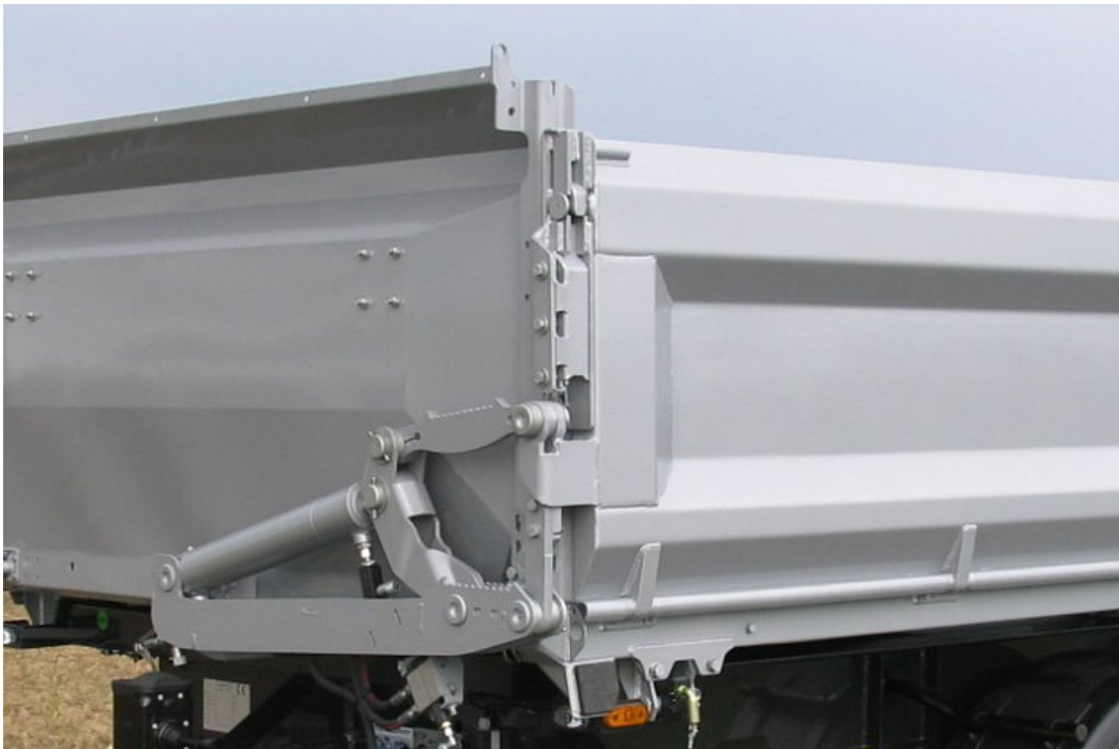
OPTIONAL: Bordmatic (= hydraulically folding side wall) on left side, with dual-action cylinder on the front wall, operated from the cab
