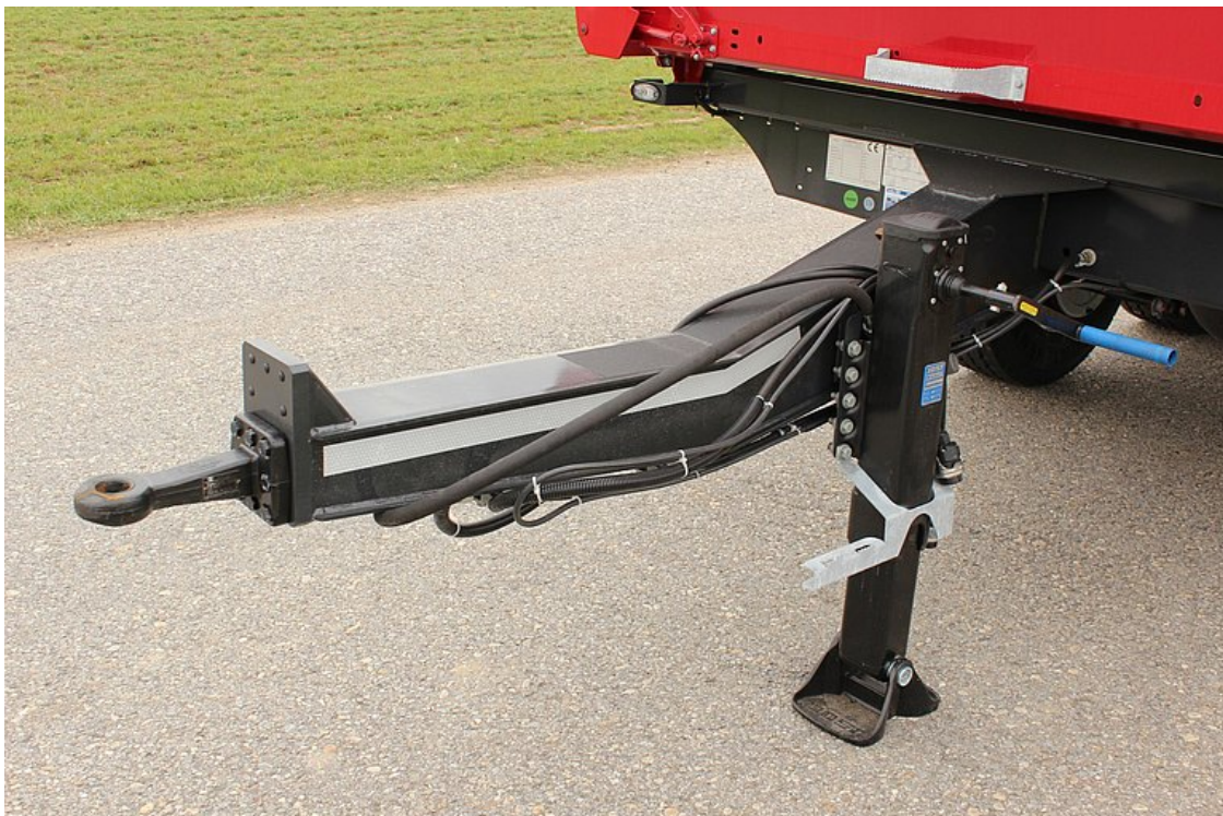
Offset drawbar with height-adjustable, screw-on drawbar eye incl. 1 step bar on the left in the direction of travel
