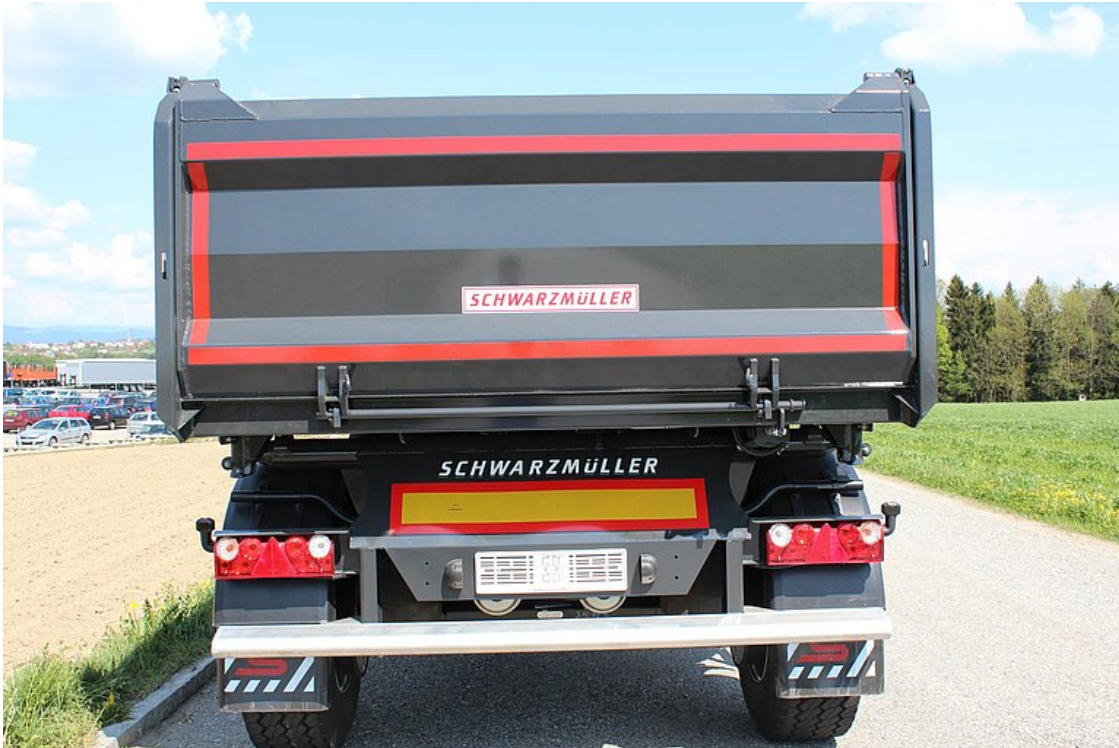
4 mm steel sheet rear wall, hinged with raised bearing and autom. pneumatic lock
