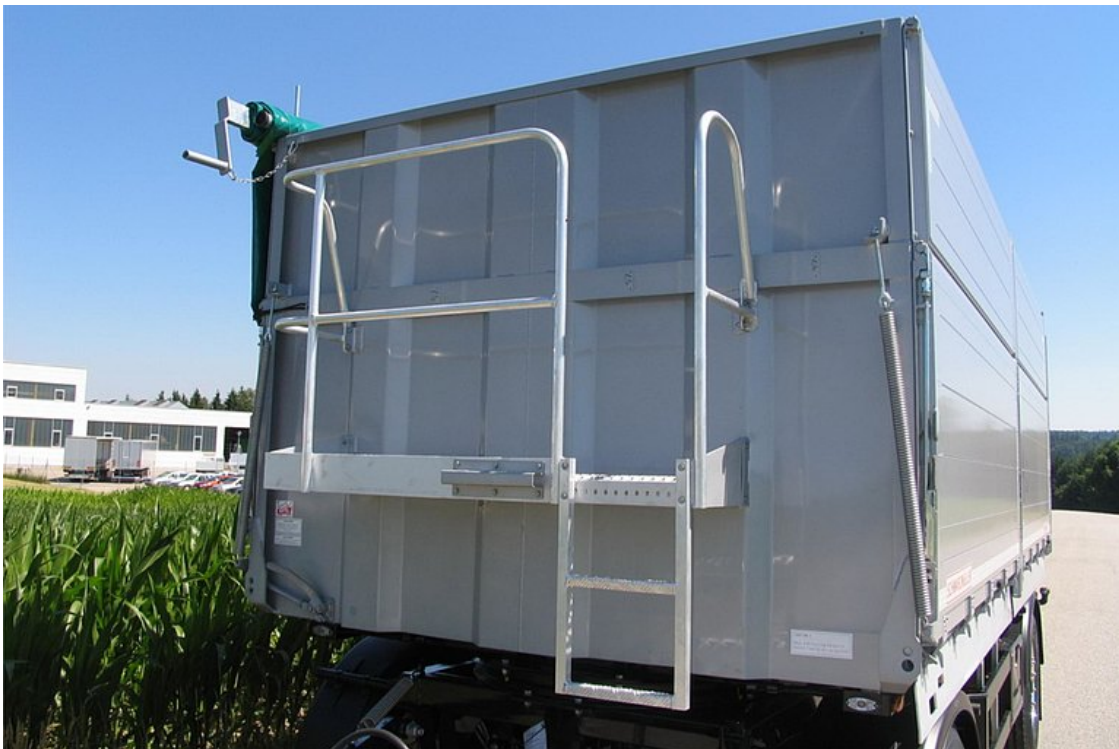
OPTIONAL: Standing platform comprising aluminium safety grid with guardrail and step unit
