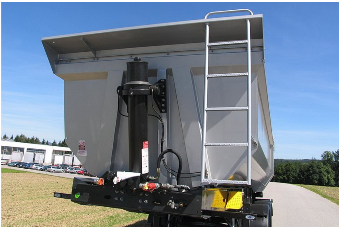
Optimum load distribution thanks to slanted front wall
