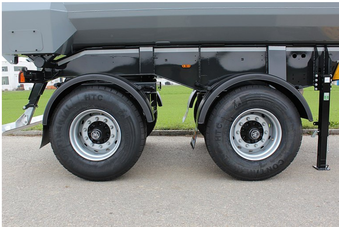
Axles with a wheelbase of 1,810 mm
