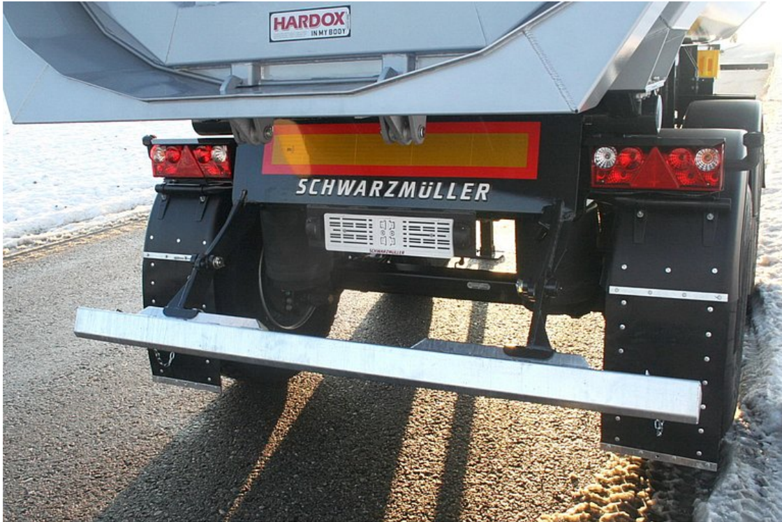
Foldable aluminium trapezoidal underride protection
