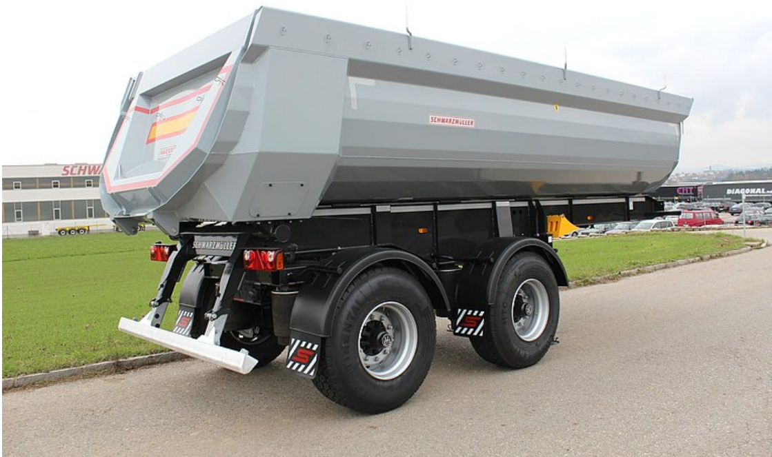
2-axle steel segment tipper semitrailer - wheelbase 1,810 mm
