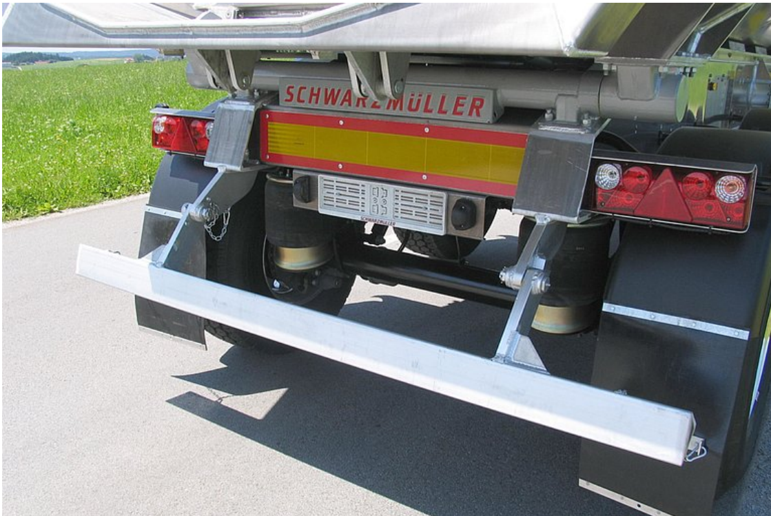
Foldable aluminium trapezoidal underride protection
