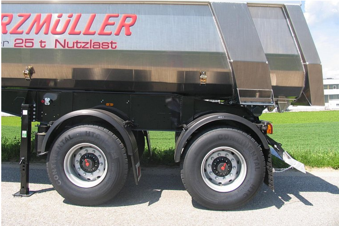
Axles with a wheelbase of 1,810 mm
