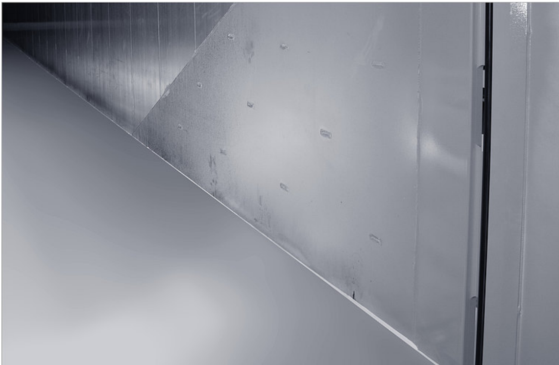
OPTIONAL: Aluminium wear plates: Reinforcements at the rear tipper box end reduce wear and therefore extend the useful life.
