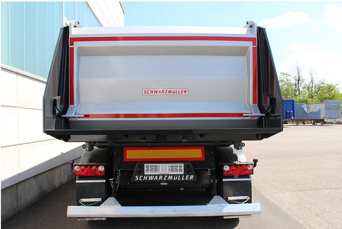
Steel sheet rear wall, hinged with raised bearing and autom. pneumatic lock
