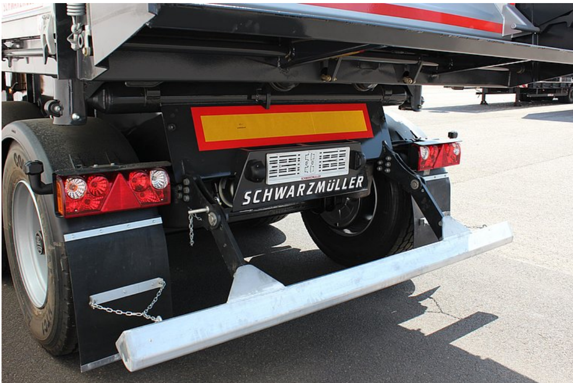
Foldable underride protection for road-finishing use
