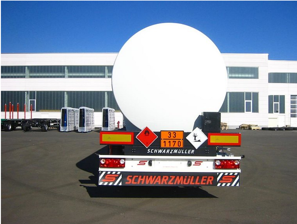
Arrangement of signage meets ADR standards
