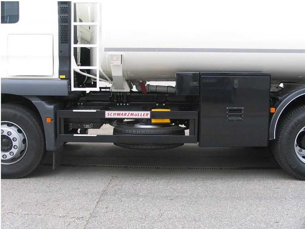
OPTIONAL: Facility for mounting spare wheel bracket
