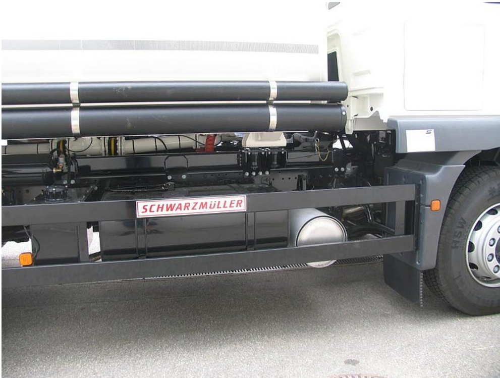
Lateral protection with aluminium profiles
