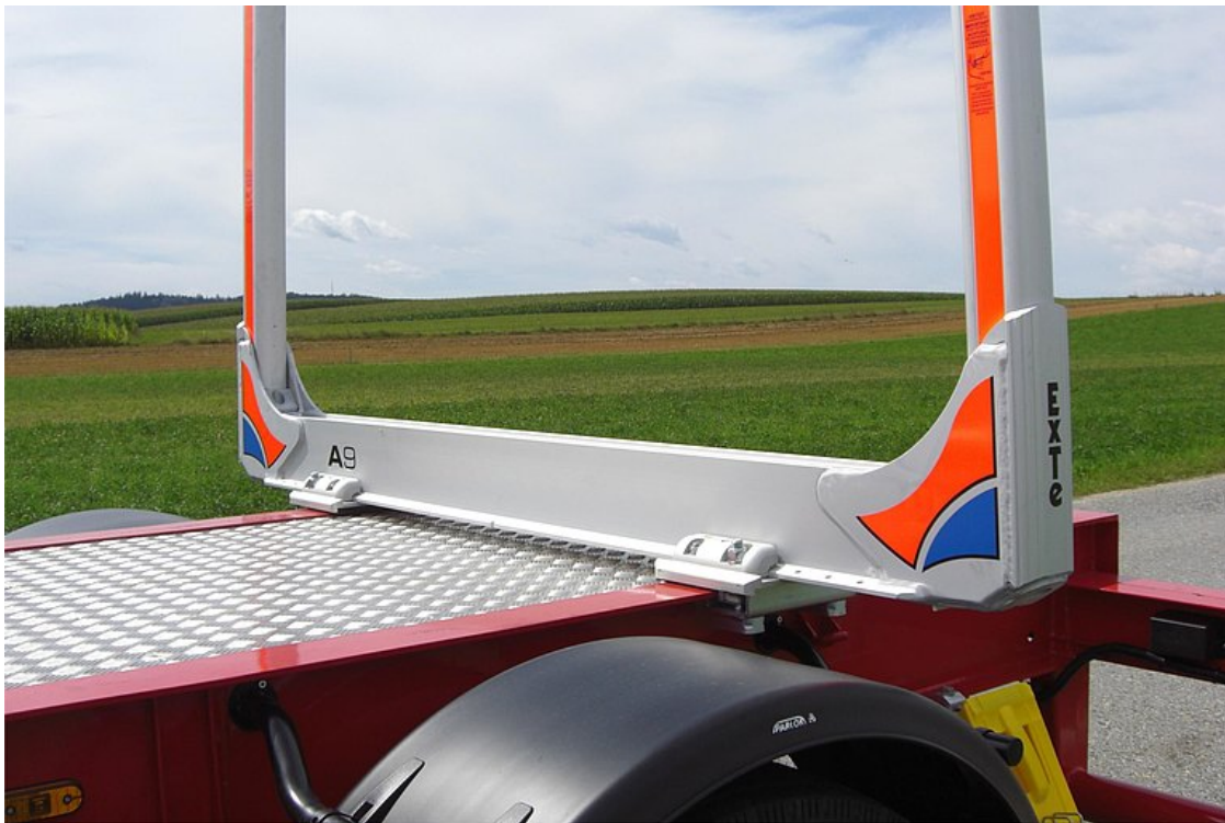
Total of 2 ExTe stanchions incl. dual-part ExTe stanchions 144 with screw attachment (loading capacity 7 t/pair)
