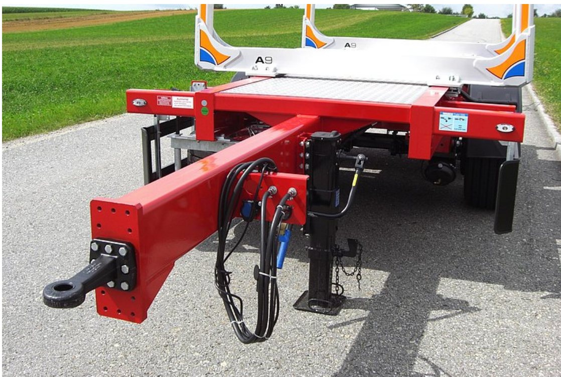
Height-adjustable drawbar for centre-axle heavy-duty coupling
