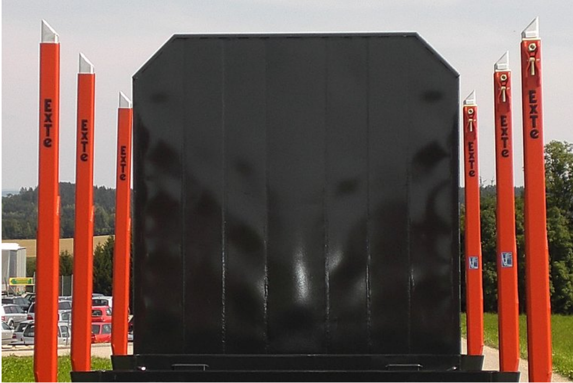
OPTIONAL: Extra-strong steel profile front wall, approx. 2,500 mm high with centre supports
