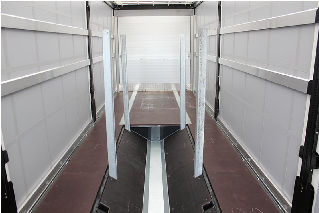
OPTIONAL: Coil recess = useful length approx. 7,400 mm - design according to VDI 2700 for coil diameters between 900 and 2,100 mm
