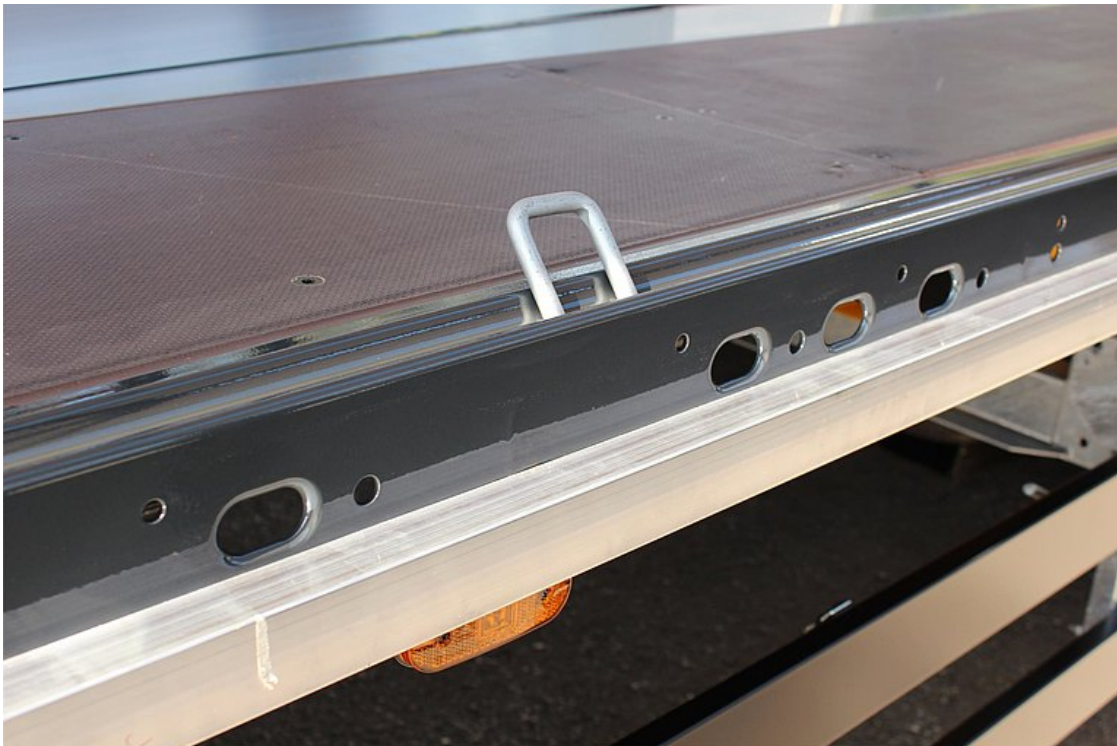
Perforated external frame (starting approx. 3,000 mm from front wall) with approx. 100 mm hole spacing, 40/25 mm slot according to DIN EN 12640 and 22 pairs of recessed 2.5 t lashing points
