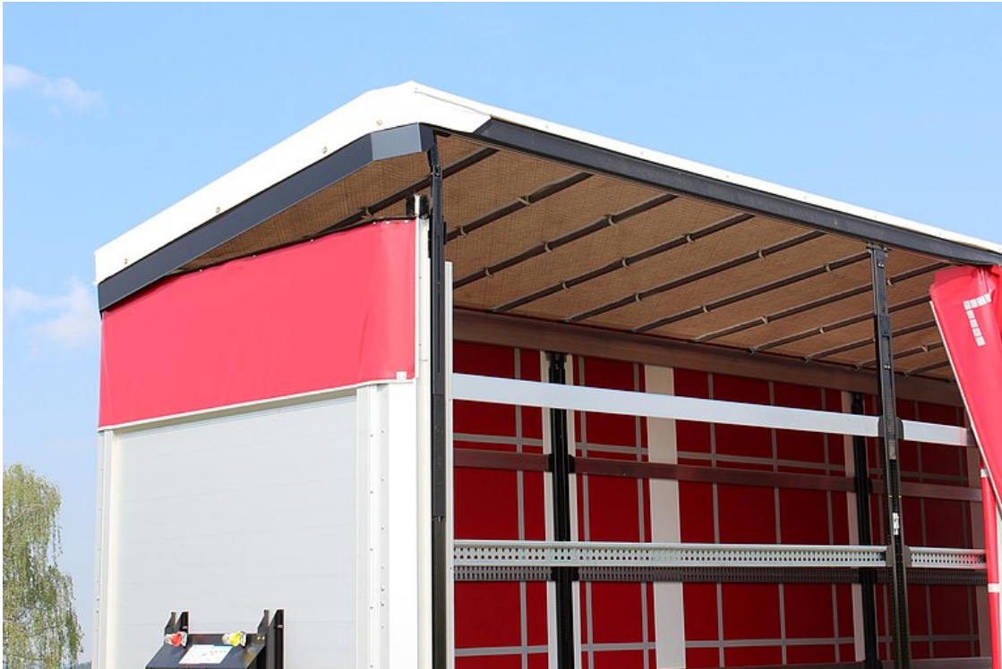
Manually operated hydraulic lifting roof, 400 mm elevation for rapid loading and unloading
