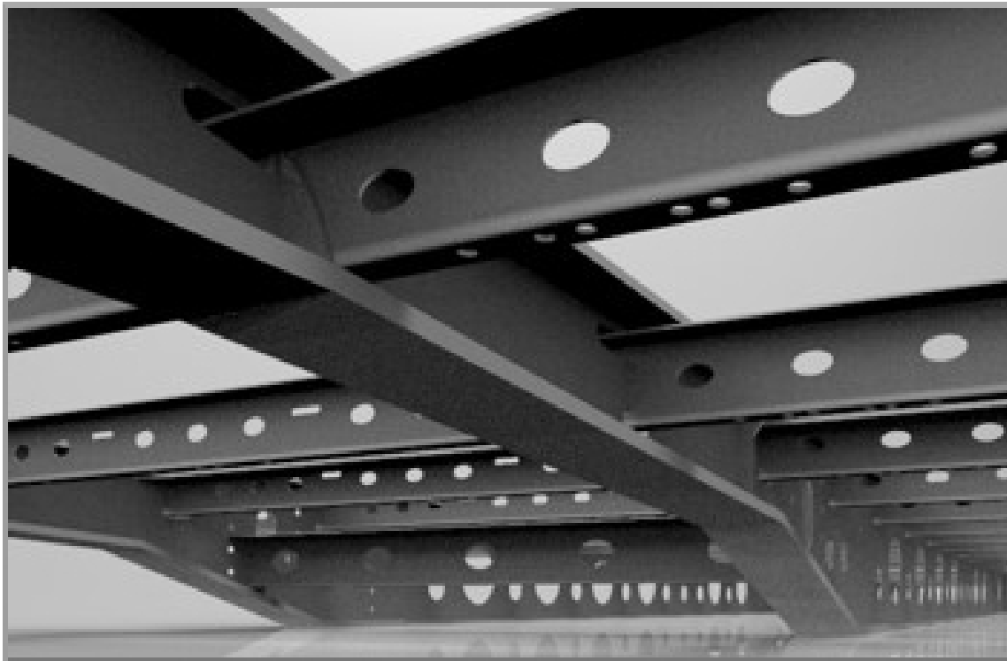
Lightweight frame: Finite element method calculations and road tests confirm its stability.
