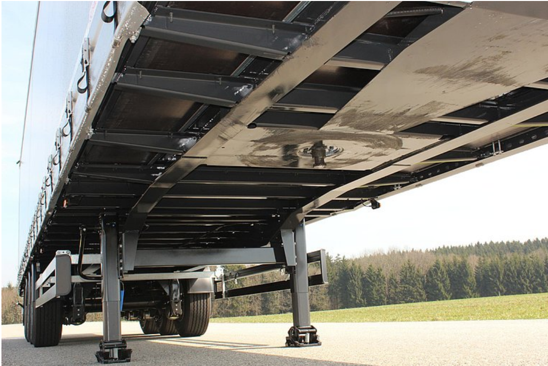
Torsionally rigid, welded ladder frame structure
