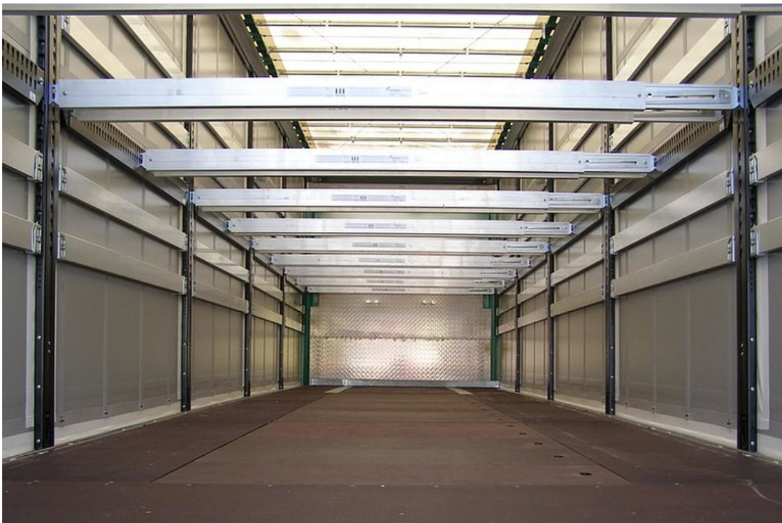
Twin-level loading system CTD for 33 Euro pallets on the 2nd loading level
