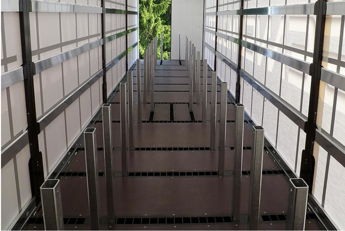
OPTIONAL: Schwarz Müller post-based load securing system with various rack positions
