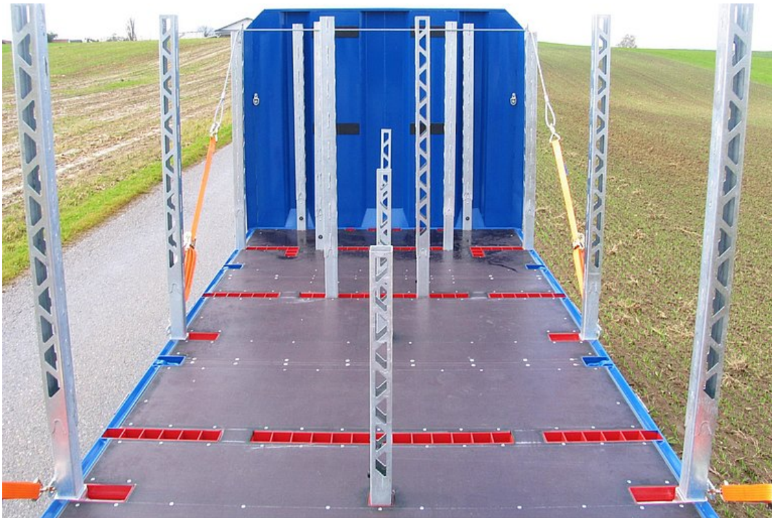
Rack positions for securing stacked construction steel mats, each with a length of 6,000 mm
