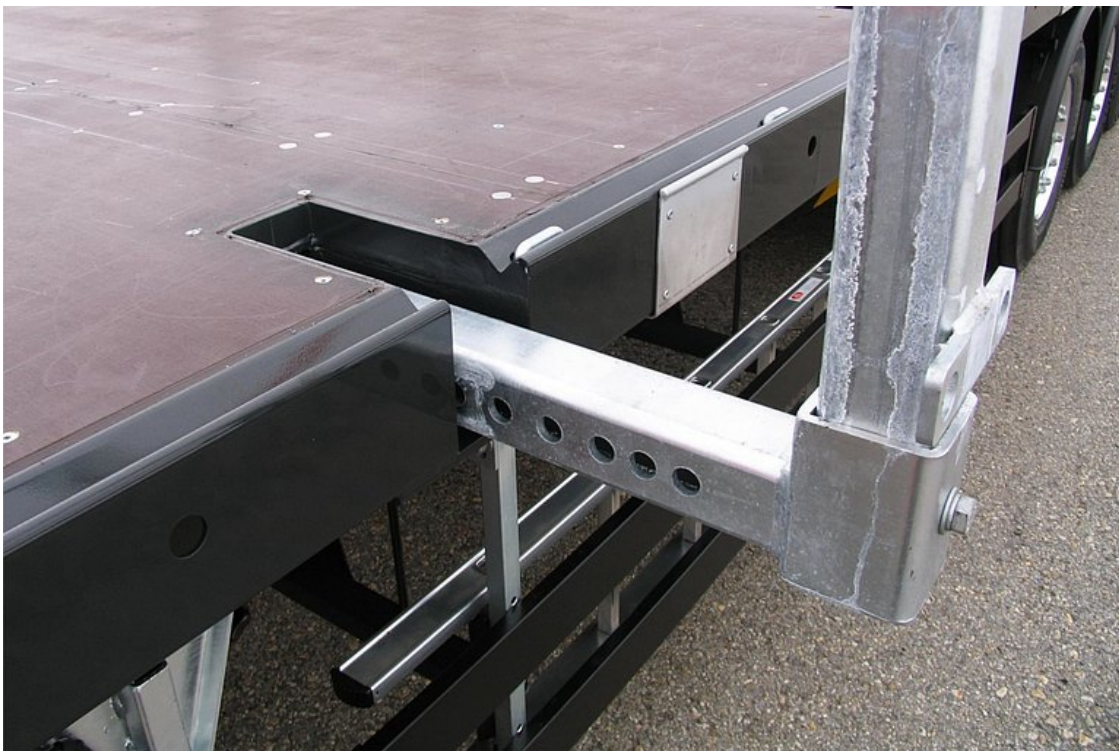
Pull-out retaining posts in lightweight tubular design, with 13 positions for load widths between 2,000 and 3,100 mm
