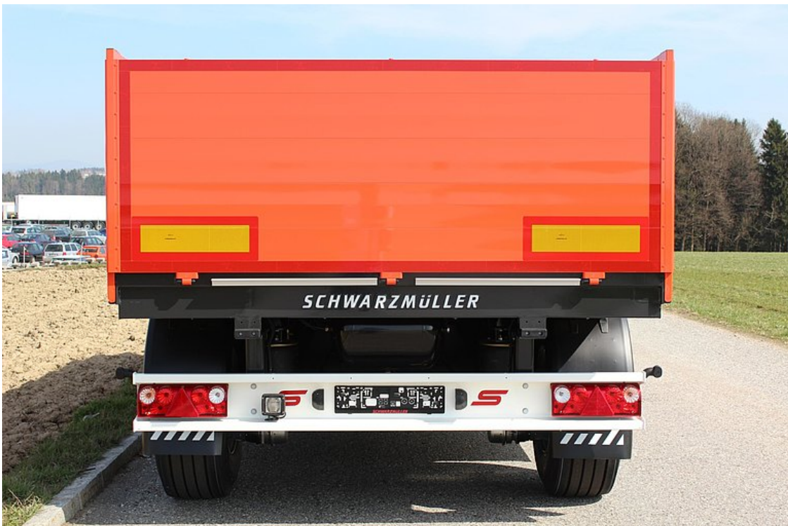
Aluminium hollow profile rear wall, internally riveted frame, foldable, with Kinnegrip double locking
