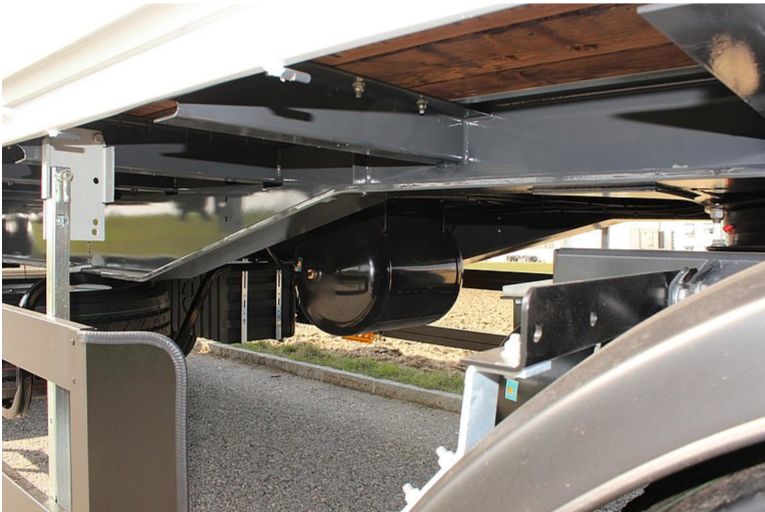
Reinforced frame design for point loading 14 t on 3 m in the centre of gravity
