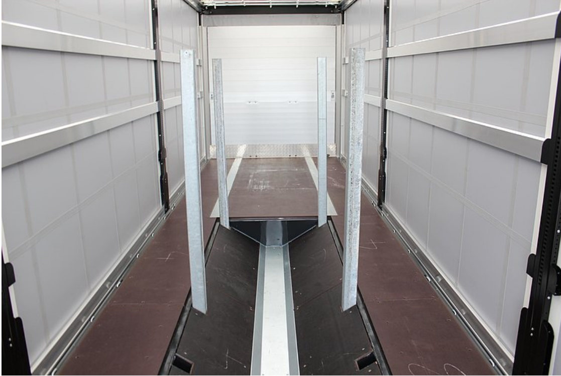
Coil recess with useful length of approx. 7,400 mm, with 5 pairs of integrated racks, for coil diameters up to 2,100 mm
