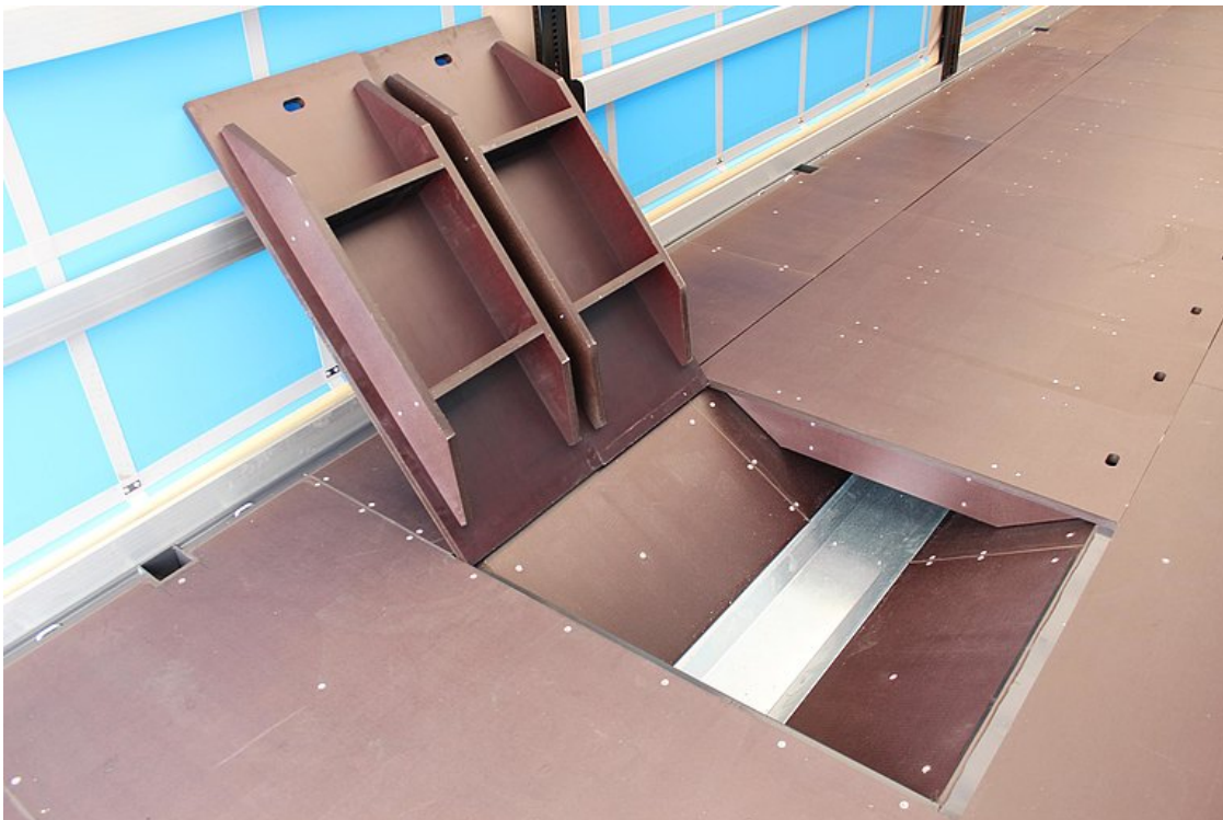
Stacker-bearing recess cover made from 27 mm resin-coated plywood with trussing
