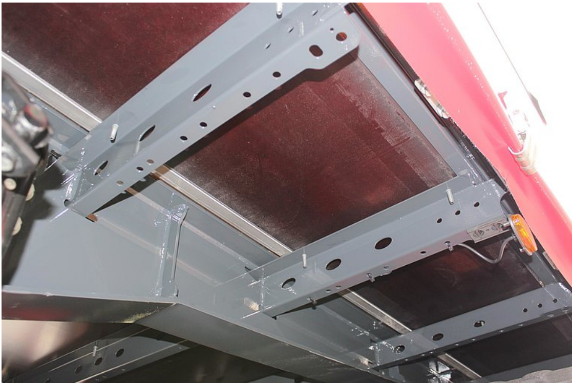
27-mm resin-coated panel floor, flush with external frame and with 2 steel top-hat profile rails above the side members (stacker axle load 7 t)
