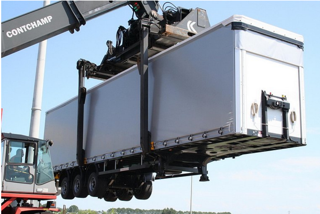
Loading example at the railway terminal
