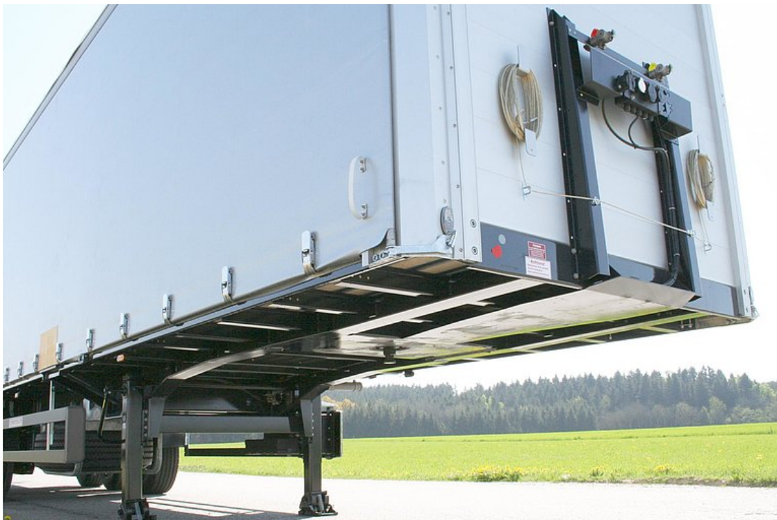
Torsionally rigid, welded ladder frame structure
