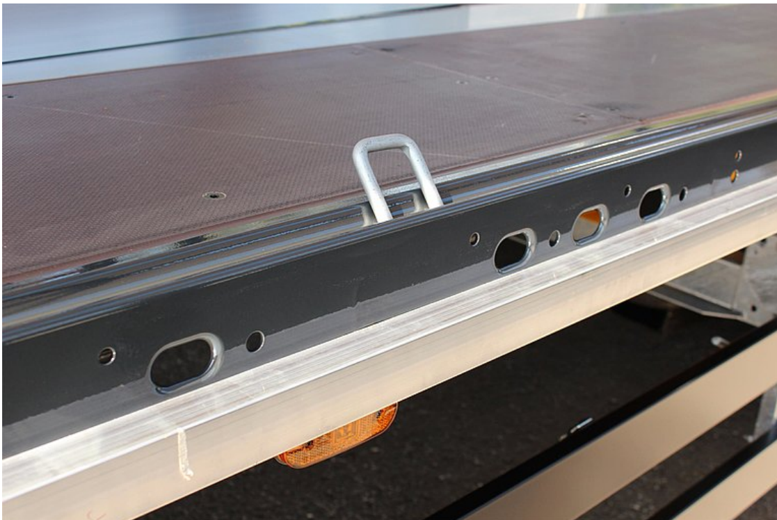
Perforated external frame with approx. 100 mm hole spacing, 40/25 mm slot according to DIN EN 12640 and 23 pairs of recessed 2.5 t
