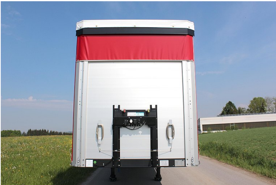
Reinforced aluminium hollow profile front wall with integrated equipment bracket
