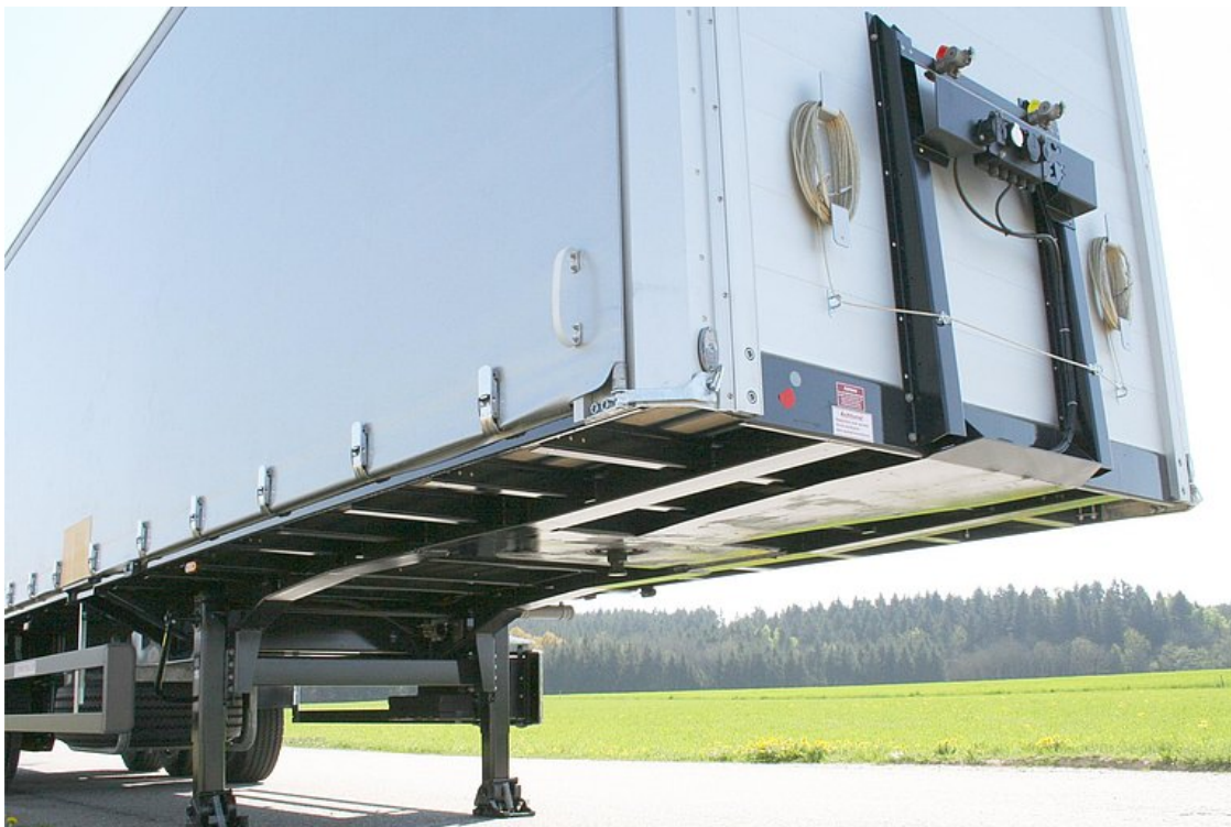
Torsionally rigid, welded ladder frame structure
