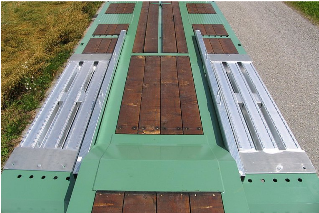
Wheel recesses with drive-on aluminium cover
