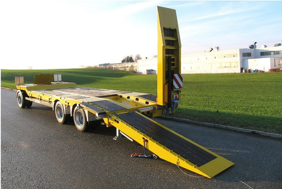
2 folding single-part loading ramps with hardwood flooring
