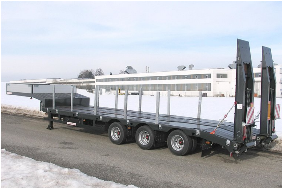
3-axle low loader semitrailer - reinforced
