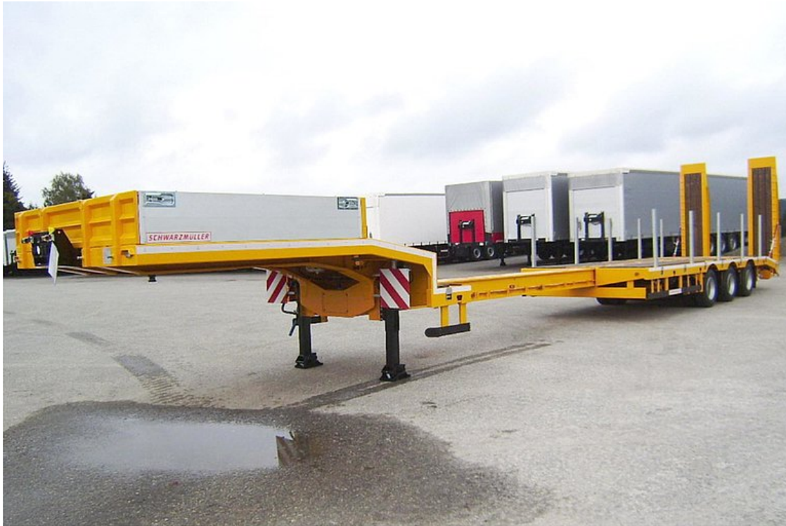
3-axle low loader semitrailer - reinforced - extendible
