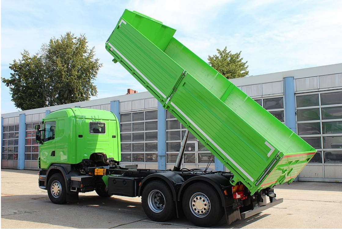
3-way tipper body on 3-axle truck - long-haul transport
