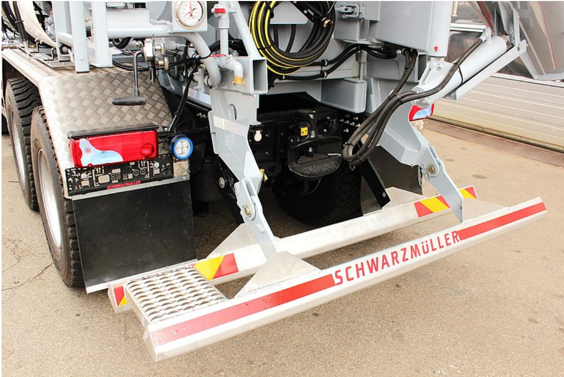
OPTIONAL: Foldable and removable underride protection
