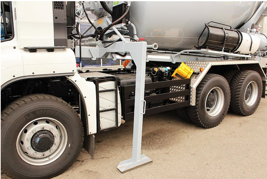
Front supports for quick and simple body replacement
