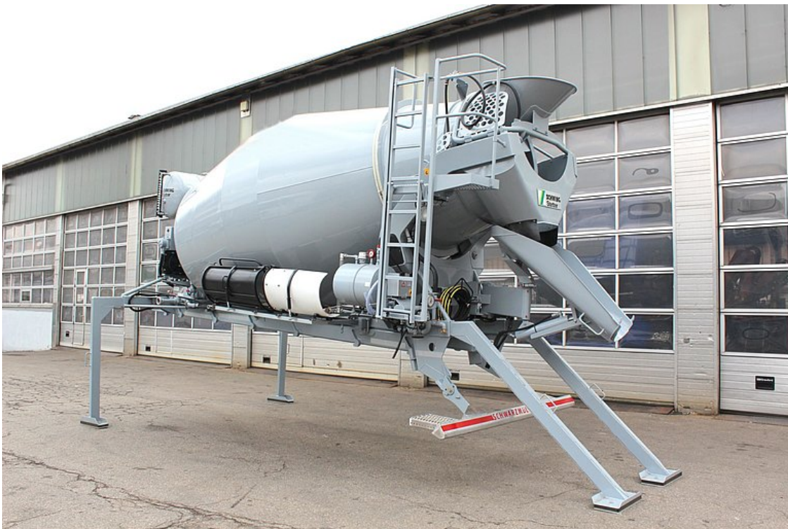
Concrete mixer body in deactivated state
