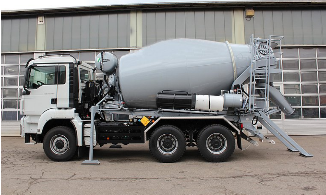
Fast-swap body system for 3-way tipper body / concrete mixer truck
