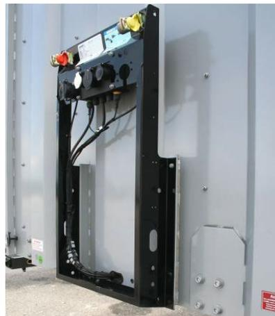
Tool holder: Check that all rivets and screws are tight
