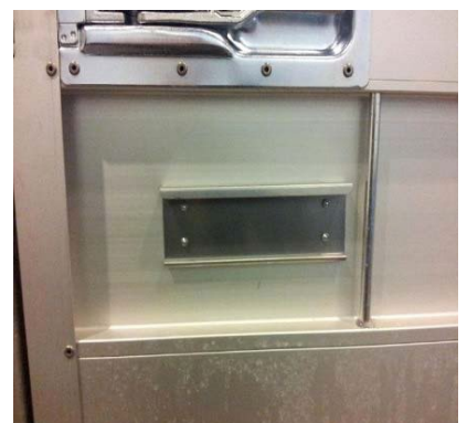
Quick-Slide latch: check that latches are tight
