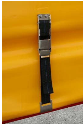
Flat hooks: Check that rivets are tight and the strap is undamaged
