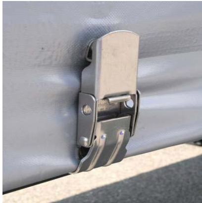
Direct tensioners: Check that rivets are tight
