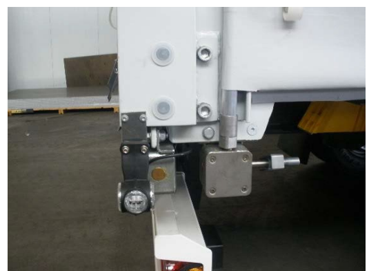
Rear tensioning gear: Check proper operation, check tarpaulin draw tube adapter for damages
