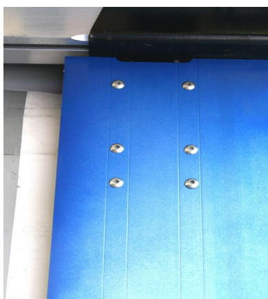
Rear corner posts: Check that rivets are tight
