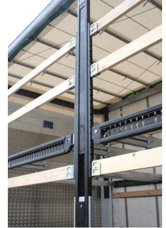
Central post: Check mounting of slat pockets
