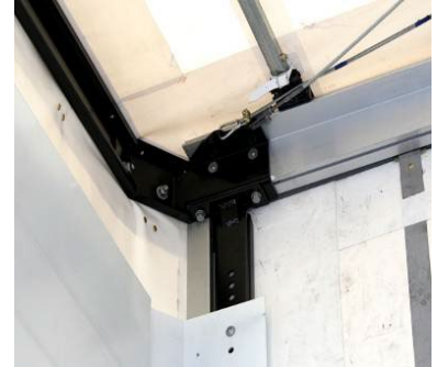
Front corner post: Check that all rivets and screws are tight
