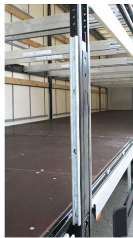
Central side posts, bottom: Check that rivets are tight
