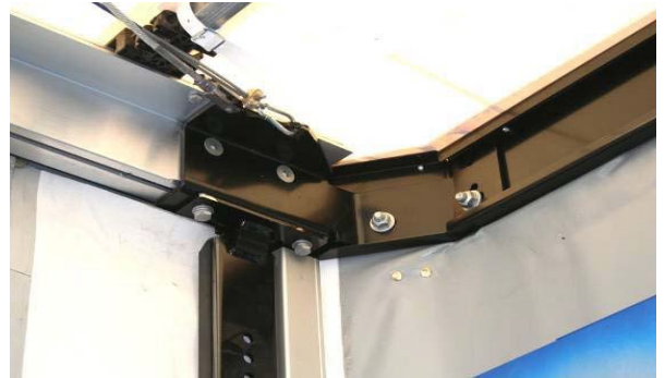
Front cover: Check that screws are tight
