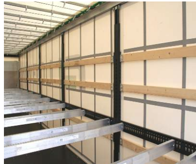
Side tarpaulin: Check the weld seams of strap reinforcements for cracks and damages
