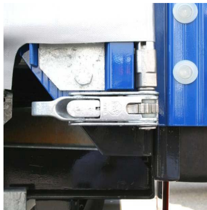
Rear tensioning gear: Check proper operability, check tarpaulin draw tube adapter for damages
