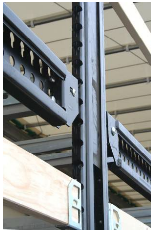
Central side posts: Check that the rail rivets are tight
