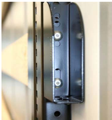
Slat pockets: Check that rivets are tight
