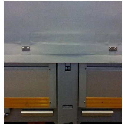
Quick-Slide tensioner: Check that rivets are tight, check belts and tensioners for damages and cracks
