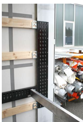
Rear corner post: Check that the rail rivets are tight
